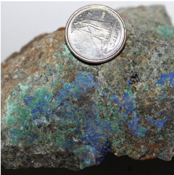
Figure 7.8 Fracture-filling azurite and malachite mineralisation in andesite porphyry rock ( J-Hf ; sample NZ003).
