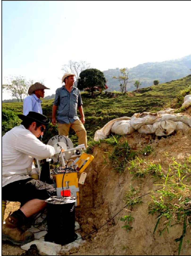
Fig 1. Technical Team on-site at Santa Elena project conduction down the hole EM survey
