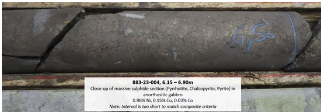
Figure 3: 883-23-004, Close-up of massive sulphide section in anorthositic gabbro
