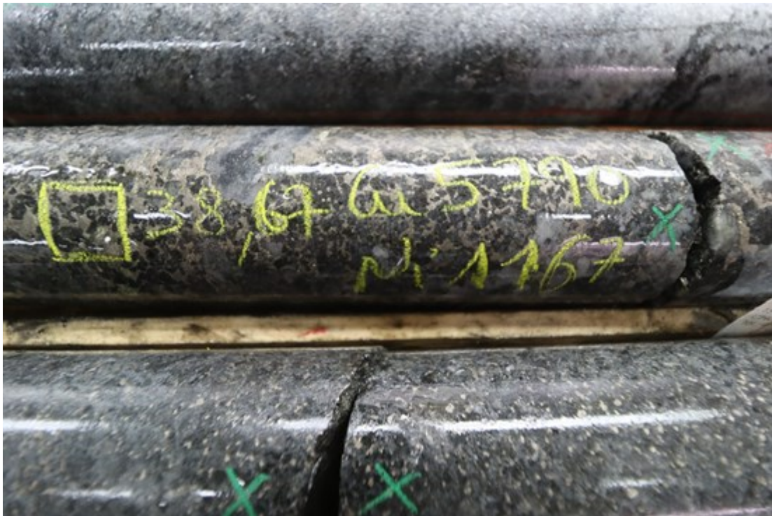
Figure 4: Hole 883-23-008, disseminated sulphide mineralization comprising pyrrhotite, pyrite, and trace chalcopyrite, which can be observed over tens of metres. Yellow marking are HH-XRF copper and nickel readings in ppm.
