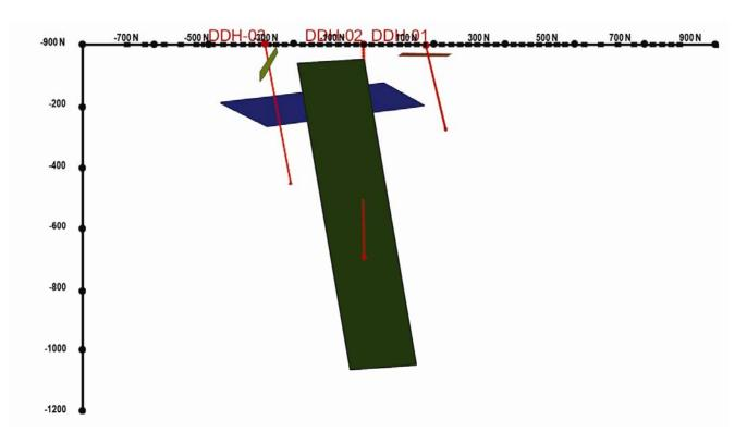
Seen in section (view towards the East) we notice the continuity at depth of the EM-03 conductor (in green), reaching more than 800 meters.
