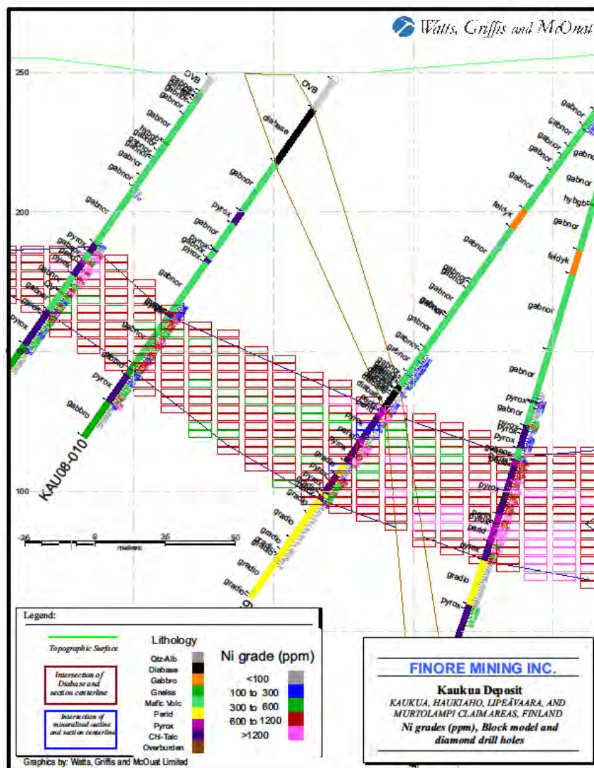
Figure 48. Vertical section showing Ni grades, block model and diamond drill holes (Kaukua)
