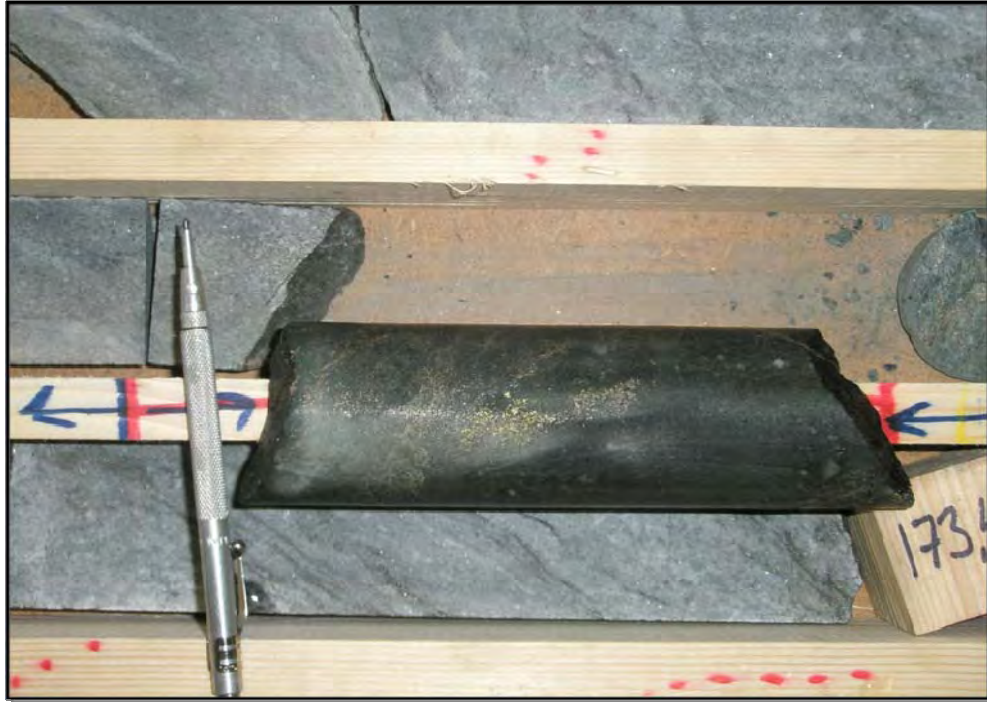
Photo 1. Photograph of sulphide mineralized drill core, Kaukua
