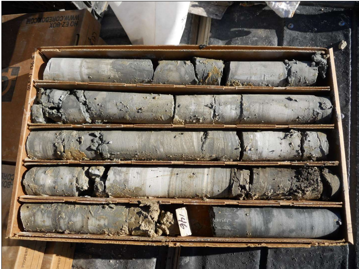
Figure 7: Lithium Mineralized Core Run from Drill Hole Solar-1 (Frank Bain Photo, 2022)
