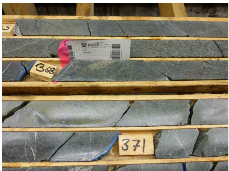
Photograph No. 12.2: Silicified and pyritic feldspar porphyry intrusive in drill hole WB-12-32 at 368.0 m
