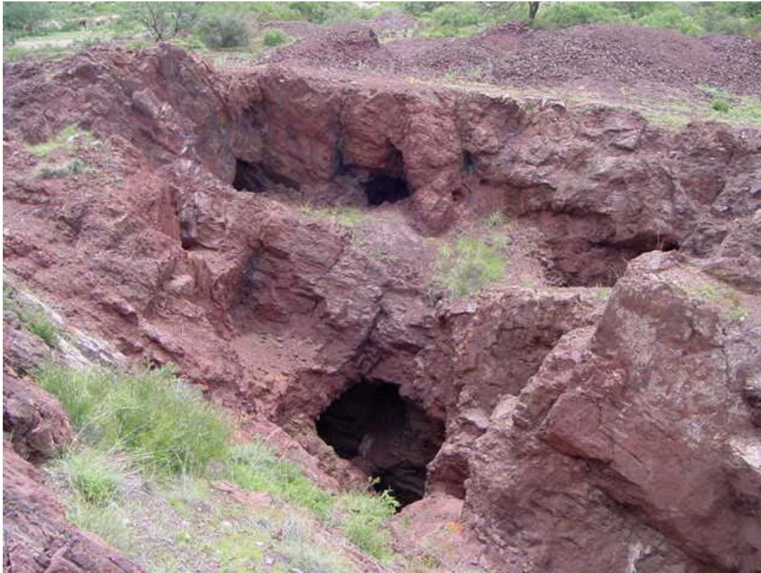
Figure 7-5 Glory Hole 2 Illustrating Moderately Dipping Massive Limestone Beds
