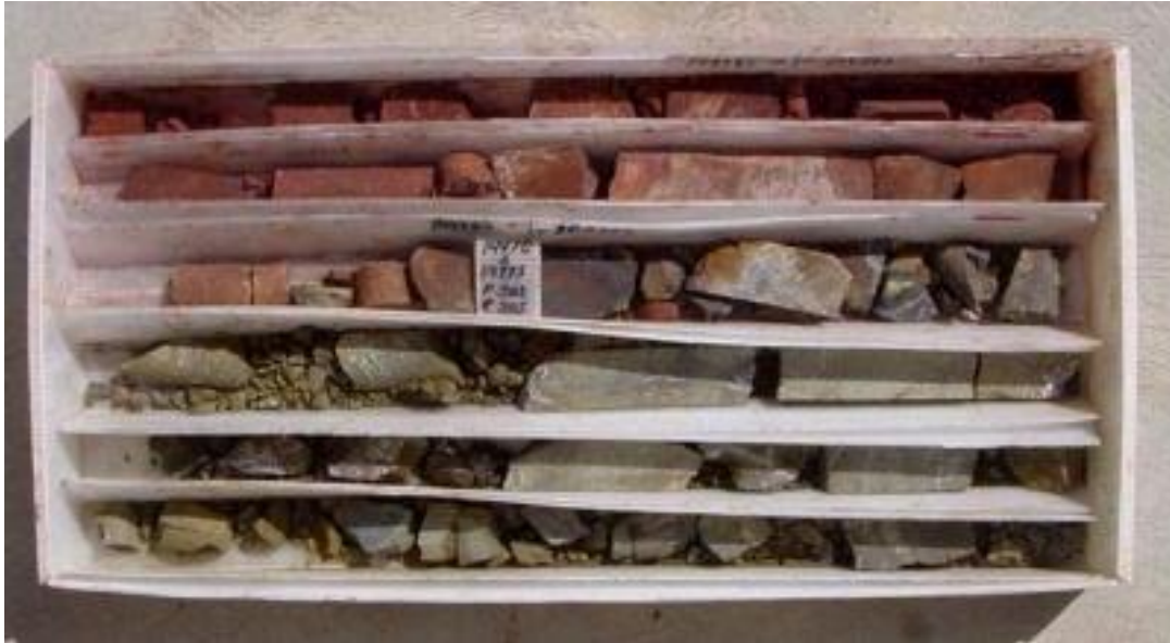
Figure 7-7 Drill Core Illustrating Oxide-Sulphide Contact (Oxide - reddish core in top half of core box Sulphide - bottom half of core box)
