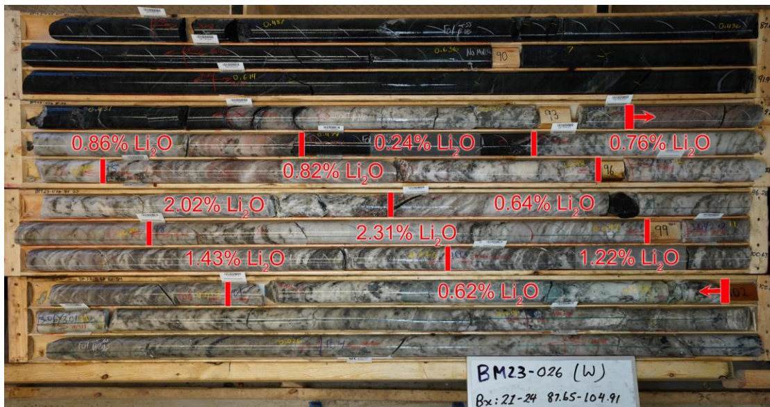
Figure 2: Core photo of hole BM23-026 (87.65 to 104.91m) highlighting \text{Li}_2\text{O} % values in high grade intercepts from 93.10 m to 102.0 m (Red).
