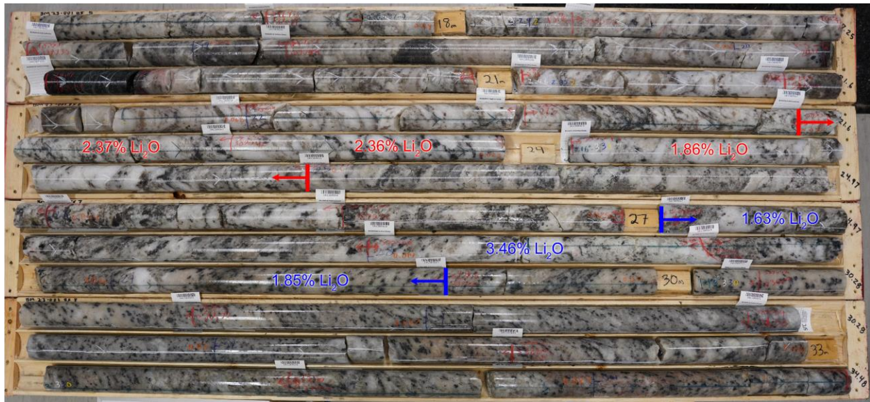
Figure 1: Core photo of hole BM23-001 (17.25m to 34.48m) highlighting \text{Li}_2\text{O}\% values in high grade intercepts from 23 -25 m (red) and 27 – 29.6 m (blue).
