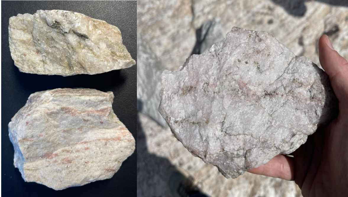
Figure 2 & 3: Example grab samples picked up at the Property showing white and pink petalite
