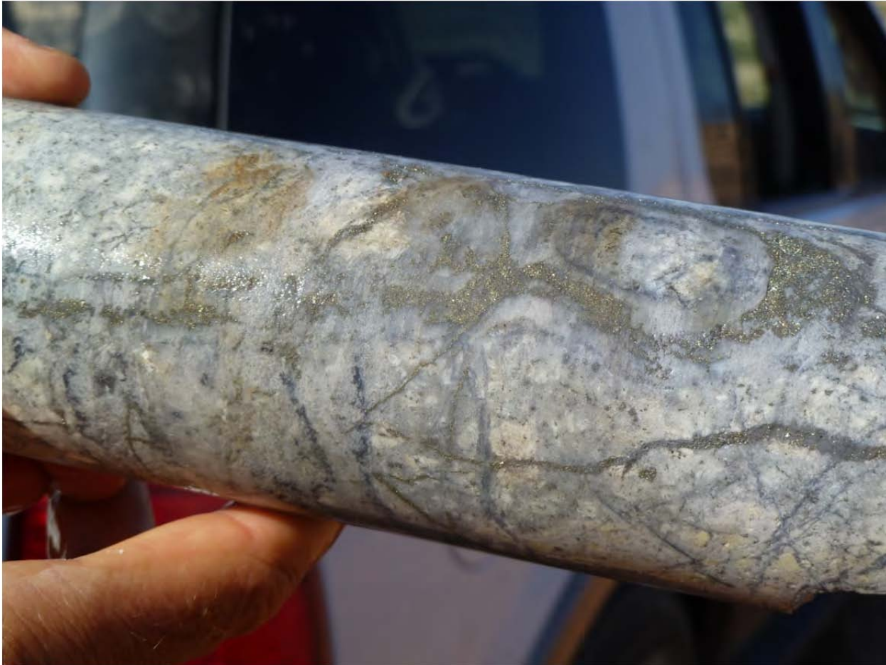
Figure 7.5 Quartz-Pyrite-Molybdenite Veinlets at Red Hills
