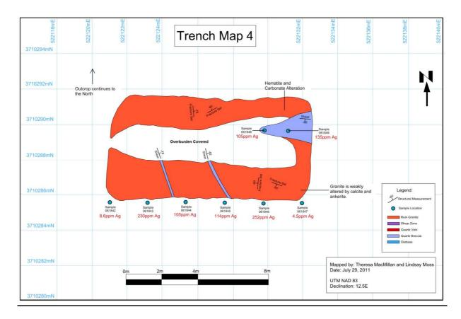
Eighty additional small trenches were mapped and sampled thoroughly in the examined area. Of the 180 samples taken 53 samples assayed over 3.2oz/t (100ppm) silver. The samples also assayed anomalous copper, lead and zinc values.
