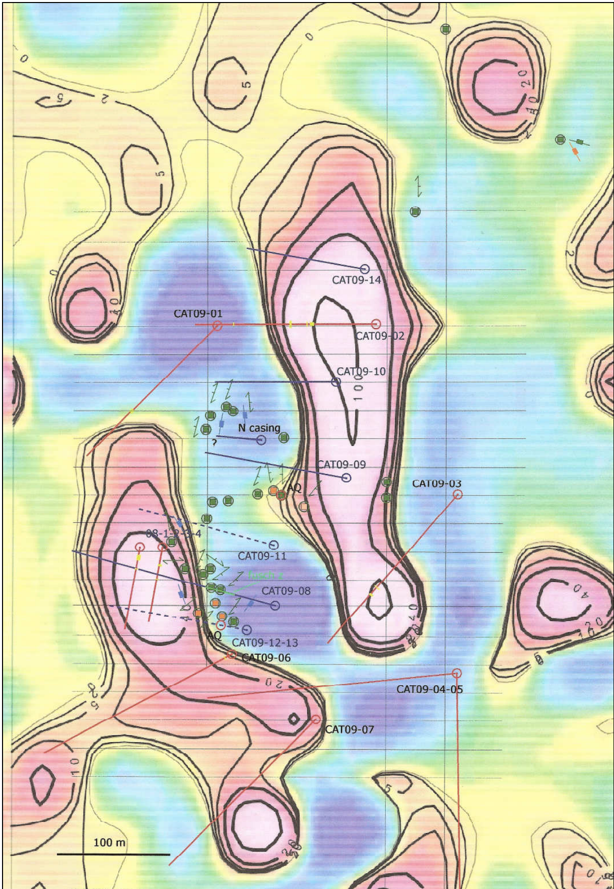
Figure 6.5.2 – Location of 2009 GDM Drillholes on VLF-EM Survey Base. Link-Catherine Property, Boston-Skead Gold Belt, Larder Lake Mining Division, Ontario (Ciesielski, 2009.
