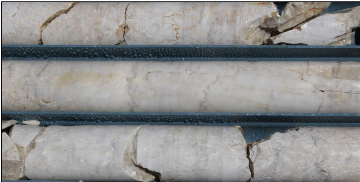
Figure 27: Bleached limestone with small-scale fluid-escape veining note pre-alteration diffuse stylolites and post-alteration open stylolite (top)
