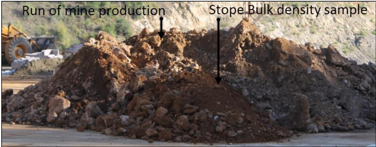
Figure 77: Stope bulk density sample # 1 and ROM production
