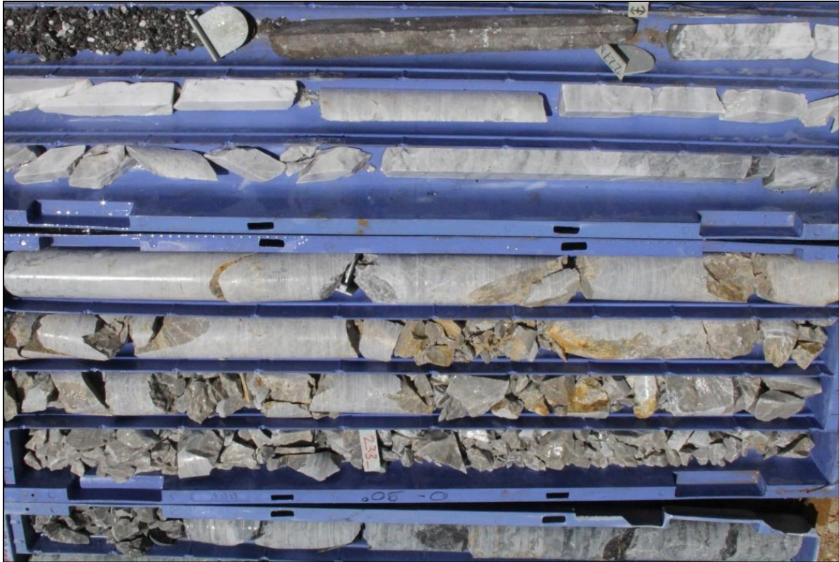
Figure 26: Massive sulphide mineralisation with thin bleached halo in footwall c. 6 m Drillhole PPS17-009 225-234 m, HQ core 63.5 mm (Source: CSA Global, 2017).
