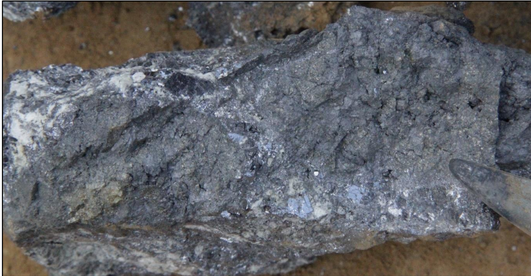
Figure 30: Massive sphalerite mineralisation veined and replaced by later galena mineralisation with iron-carbonate gangue; stockpile sample
