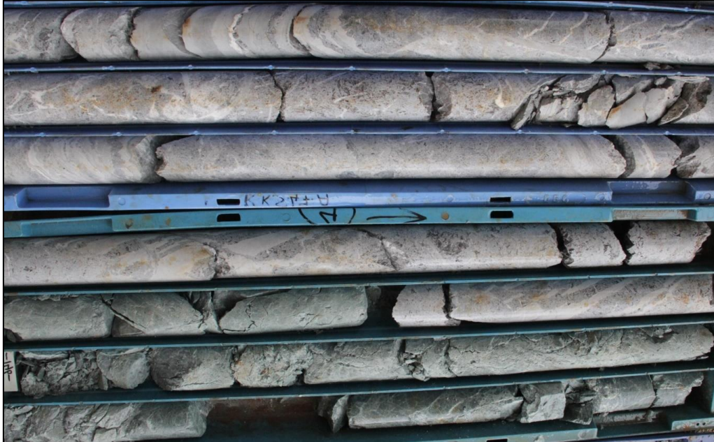
Figure 23: Basal contact of the Değirmentaş Formation altered veined limestone and bleached siltstone horizons. Note sharp contact down into green chloritic micro-brecciated tuffaceous unit. Drillhole PPS17-004 141-147 m, HQ core 63.5 mm (Source: CSA Global, 2017).
