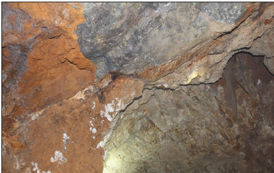
Figure 32: Massive sulphide with stratabound contact with bedded grey limestone, cut by oxide mineralisation that also cuts across the limestone in a karstic feature; Pinargozu mine
