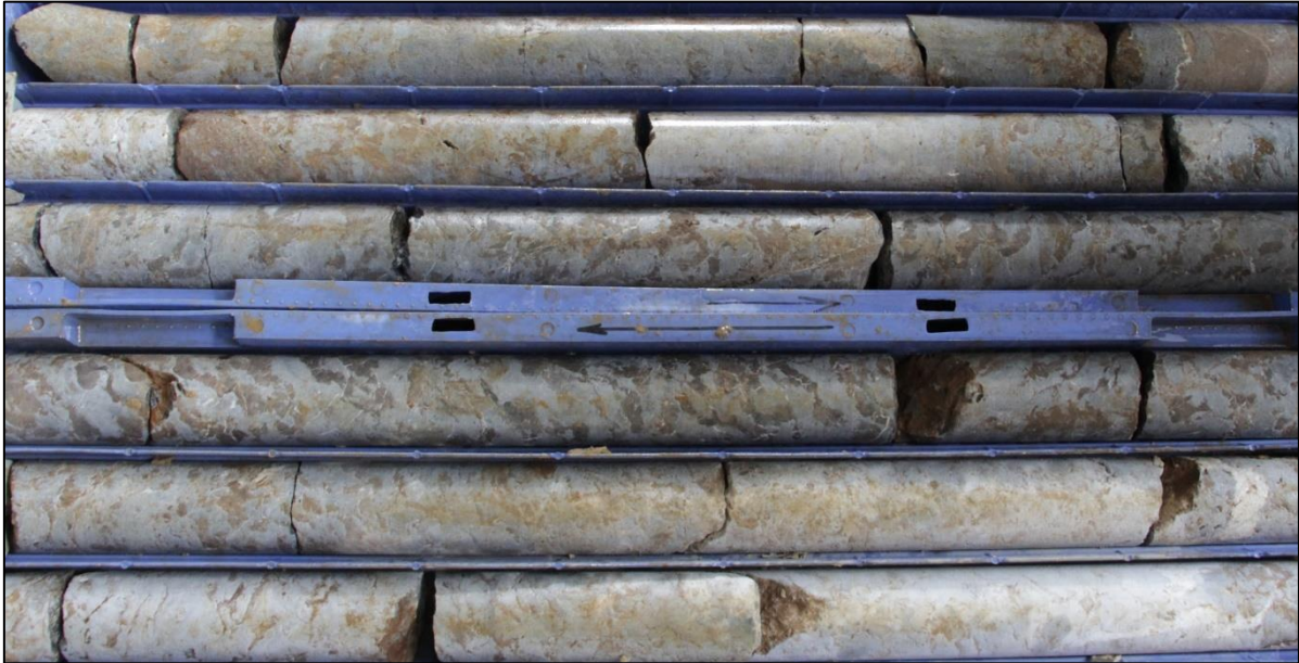
Figure 19: Lower Değirmentaş Formation, distinctive lower unit of blotchy bioturbated limestone that occurs in the mineralisation footwall, with partial bleaching
