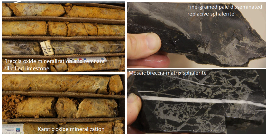
Figure 1 Left image - High-grade zinc oxide mineralization from drill hole SRDD-2018-001. Right image - Fine grained, low-iron sphalerite in black shale from drill hole SRDD-2018-004
