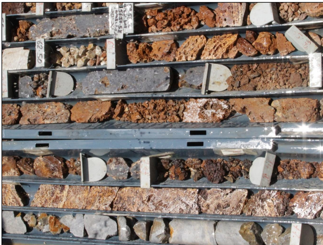
Figure 34: Remnant massive galena mineralisation in high-grade smithsonite oxide zinc ore Drillhole PPU16-042 52-77 m, HQ core 63.5 mm (Source: CSA Global, 2017).
