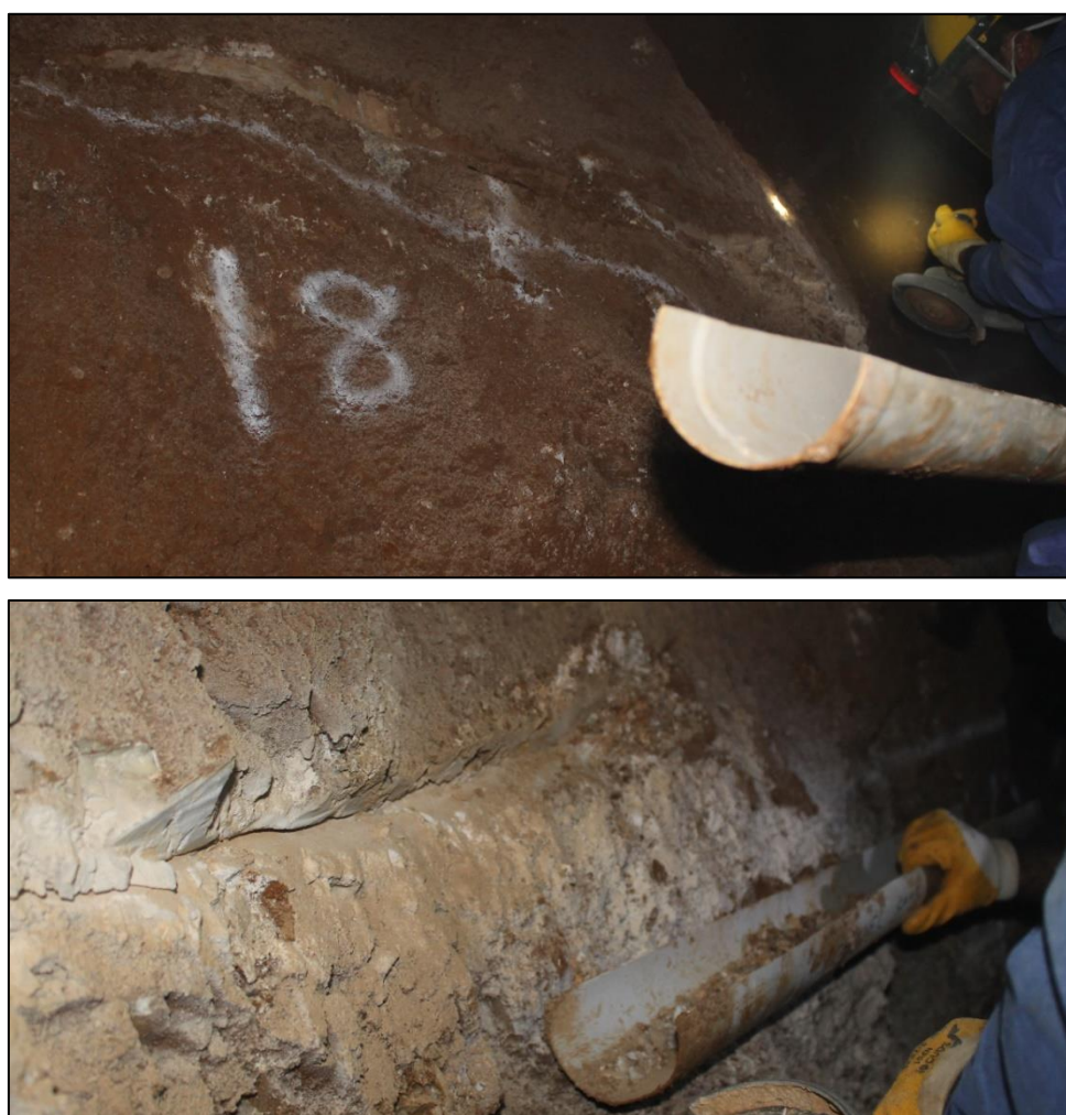
Figure 45: Channel samples being collected with a rock saw and half-pipe (Source: Pasinex, 2017)
