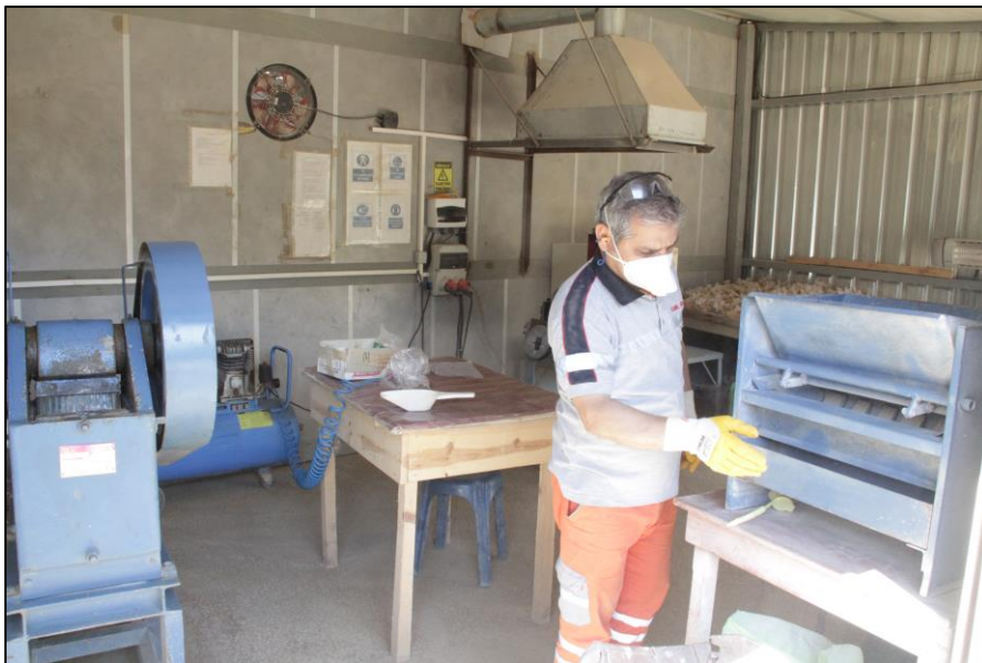
Figure 46: Jaw crusher and riffle splitter at Horzum
