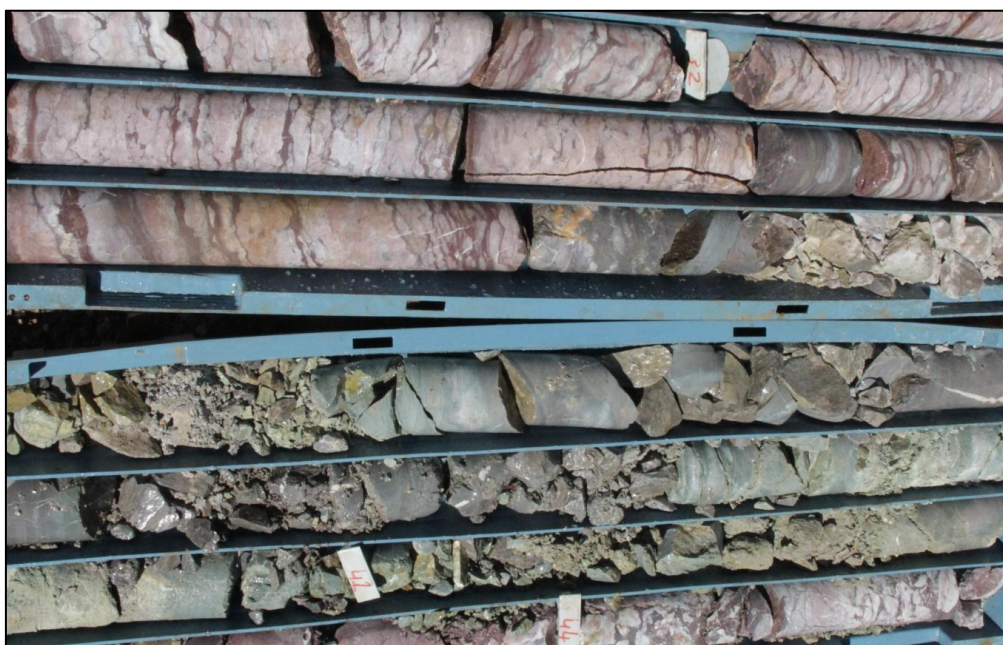
Figure 22: Upper Değirmenteş Formation nodular argillaceous limestone, reddish, with horizons of green siltstone
