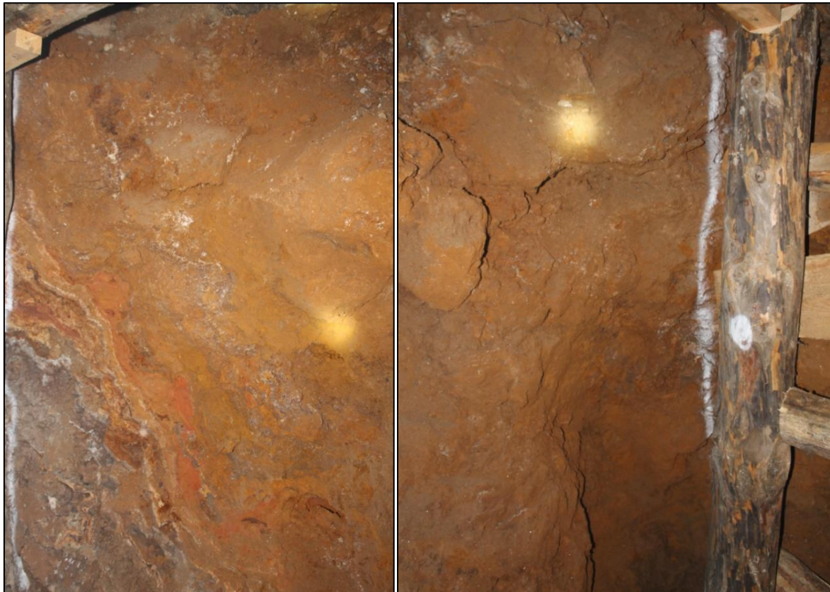
Figure 78: Underground face selected for stope bulk density, before blasting
