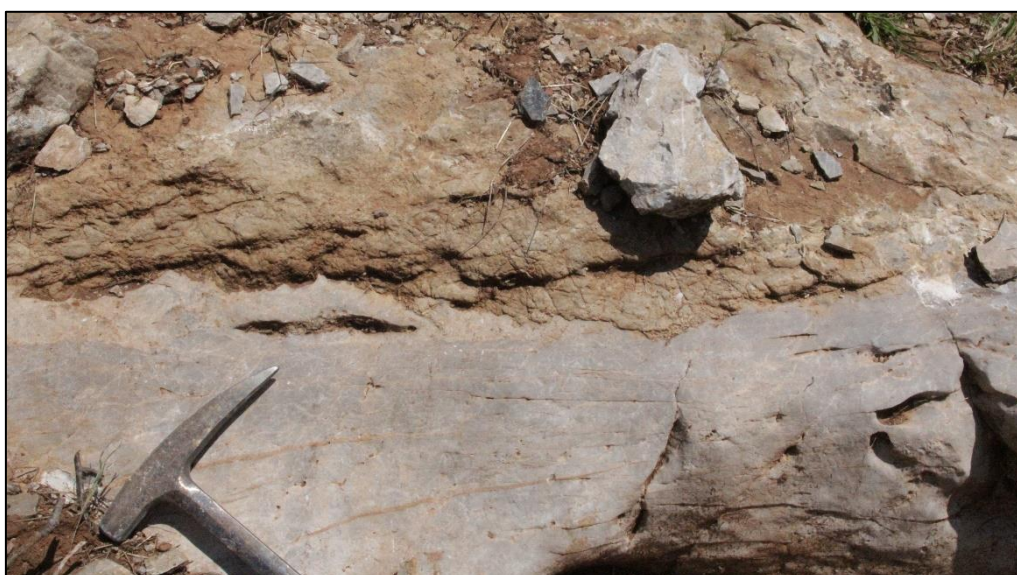
Figure 24: Contact between grey micritic limestone and brownish dolostone Değirmentaş Formation at Akkaya (Source: CSA Global, 2017).
