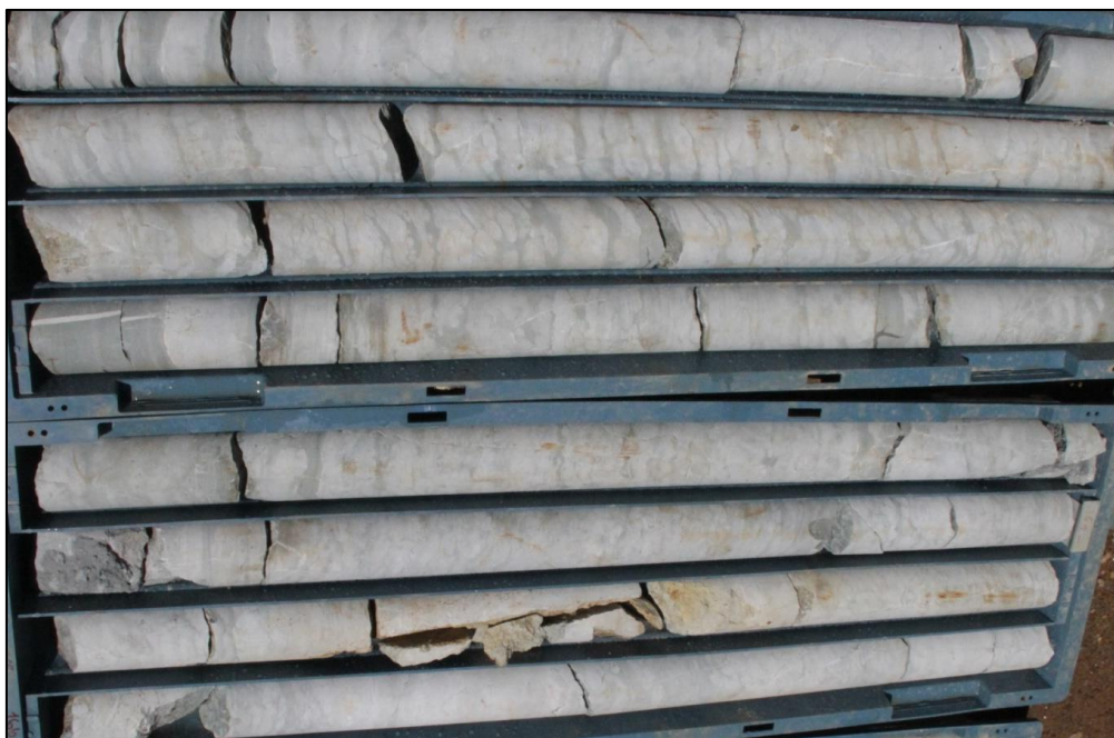
Figure 21: Upper Değirmenteş Formation nodular argillaceous limestone and minor siltstone down into nodular and massive limestone
