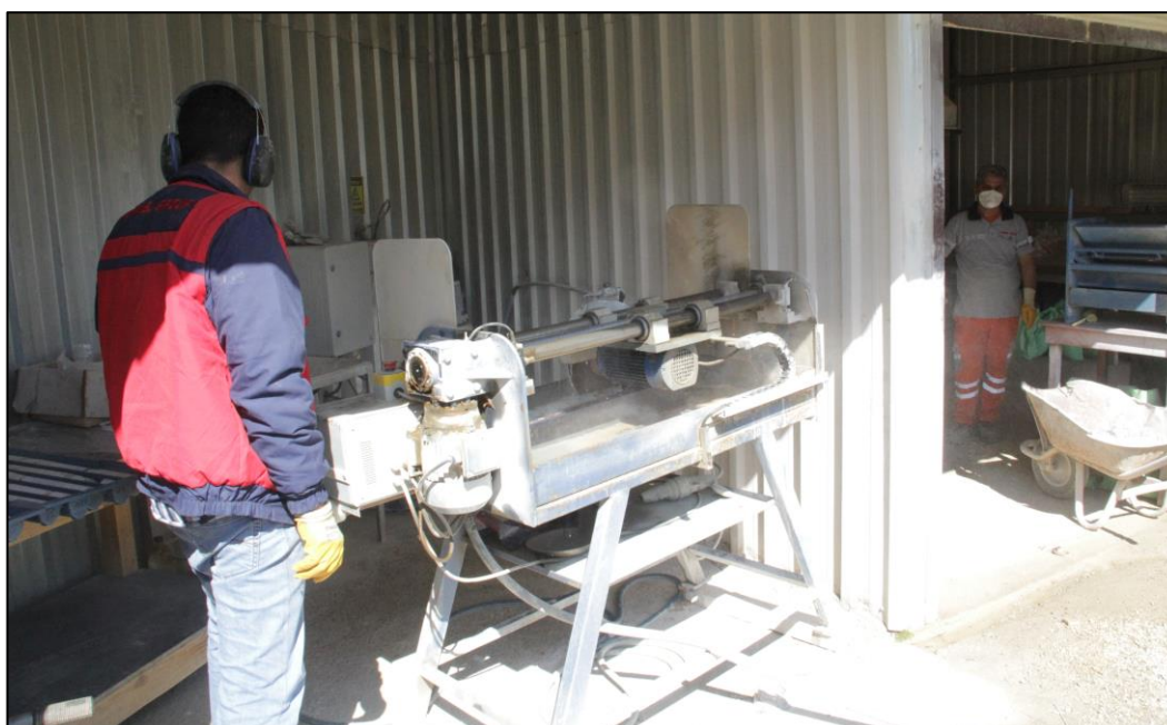
Figure 44: Drill-core cutting at Horzum
