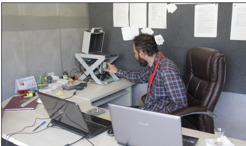
Figure 48: pXRF sample pulp screening at Horzum
