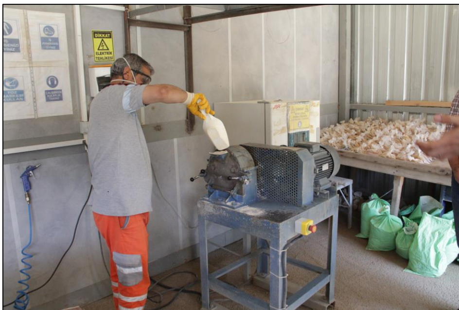
Figure 47: Pulverising crushed sample with a disc mil, Horzum
