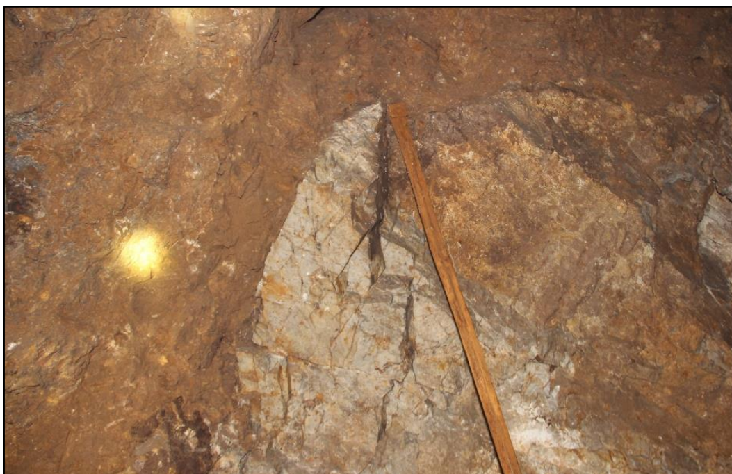
Figure 35: Sharp contact of secondary karstic zinc mineralisation with bleached bedded limestone Note that the contact is irregular and dissolution-related and is not a fault; Pinargozu mine (Source: CSA Global, 2017).
