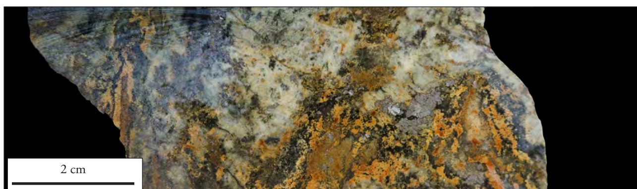
Figure 20: Chlorite-epidote alteration overprinted by silica and blebby, massive arsenopyrite. From a 1.40 metre interval which assayed 4.52 ppm gold. 125.1 to 126.5 metres, PA-1.
