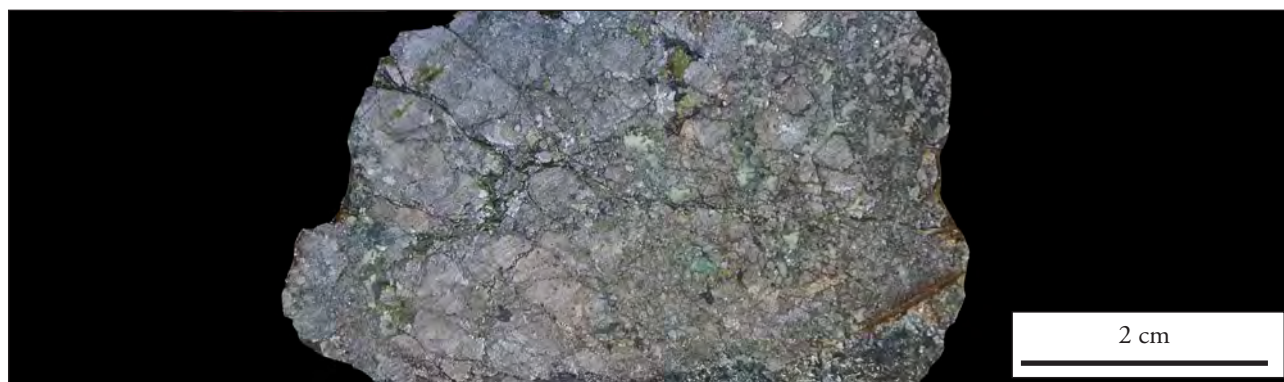
Figure 22: Massive, strongly fractured arsenopyrite with minor intergrowths of pyrite and galena. From a 1.9 metre interval which assayed 3.73 ppm gold, 92 ppm silver, 0.19 % copper, 3.61 % lead and 1.21 % zinc. 172.6 to 174.4 metres, PA-1.
