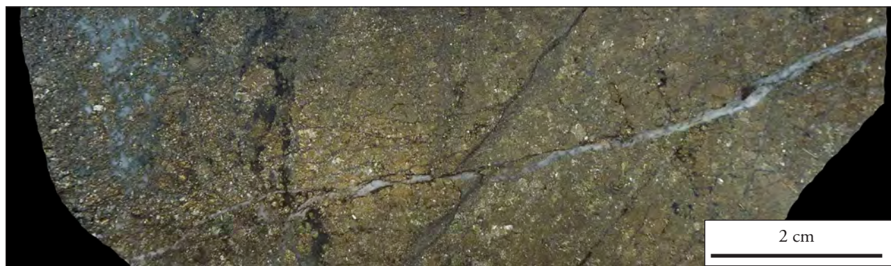
Figure 21: Massive, strongly fractured and friable pyrite and trace chalcopyrite with interstitial pale grey quartz, fine-grained galena and chlorite in fault zone. Sinistrally offset by calcite veinlet. From a 1.7 metre interval which assayed 0.14 ppm gold, 97 ppm silver and 0.27 % copper. 358.3 to 360.3 metres, PA-1.
