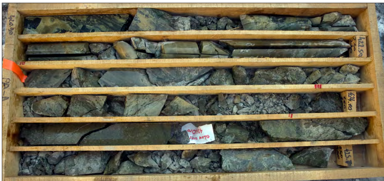
Figure 24: Altered interbedded sedimentary rock crosscut by massive sulphide hosted in a fault zone (424.0 to 424.5 metres), marked by strong fracturing of the wall rock at the hanging and footwall contacts. Core box contains core from 420.9 to 425.7 metres, PA-1.
