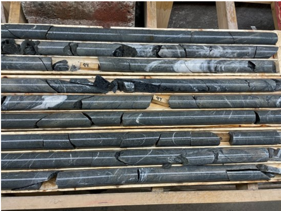
Figure 2 - Brittle-Ductile shearing in Zone A hosting quartz-carbonate (chlorite) veining. Section of core from RSG-21-068 that grades 5.00m @ 7.25 g/t Au (92.85 - 97.85m).
