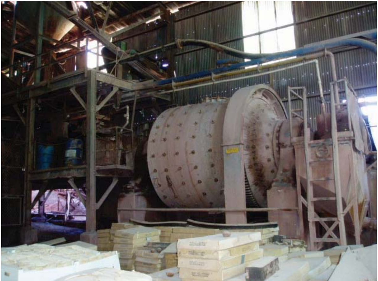
Figure 6.2 Atlanta Mill - Ball Mill
