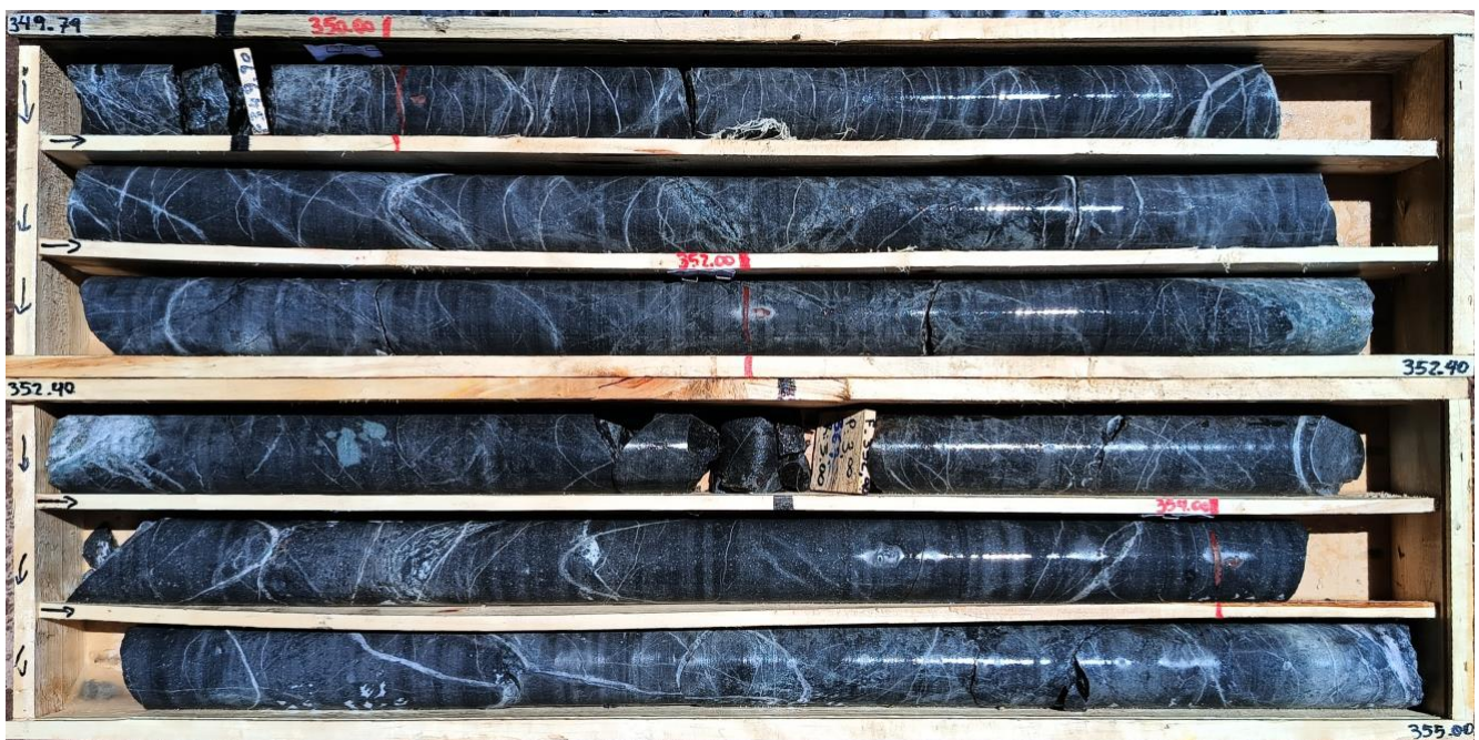
Image 4: PIU-04 349.79 – 355.0 m. Volcanic andesite host rock with strong biotite-magnetite alteration and consistent quartz-sulfide veining.
