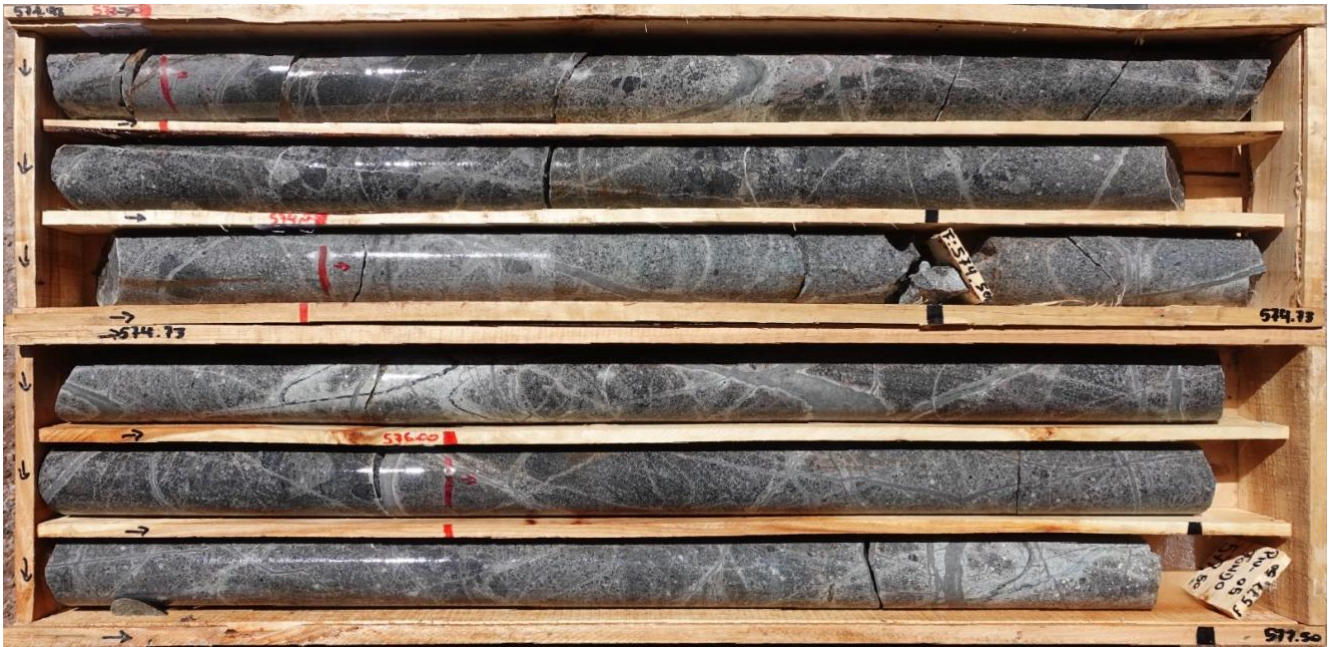
Image 2: PIU-05 571.9 - 577.5m. Strongly veined and porphyry and diorite host rock and intercalated quartz-porphyry, showing multiphase quartz A-veins and associated K-feldspar bearing potassic alteration.
