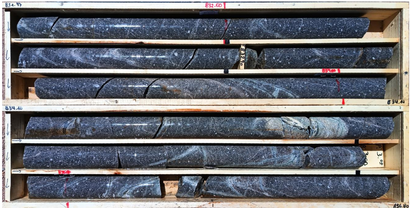
Image 5: PIU-04 834.47 – 836.80 m. Strongly biotite-magnetite altered pre-mineral diorite porphyry with moderate intensity quartz porphyry style A-veins.
