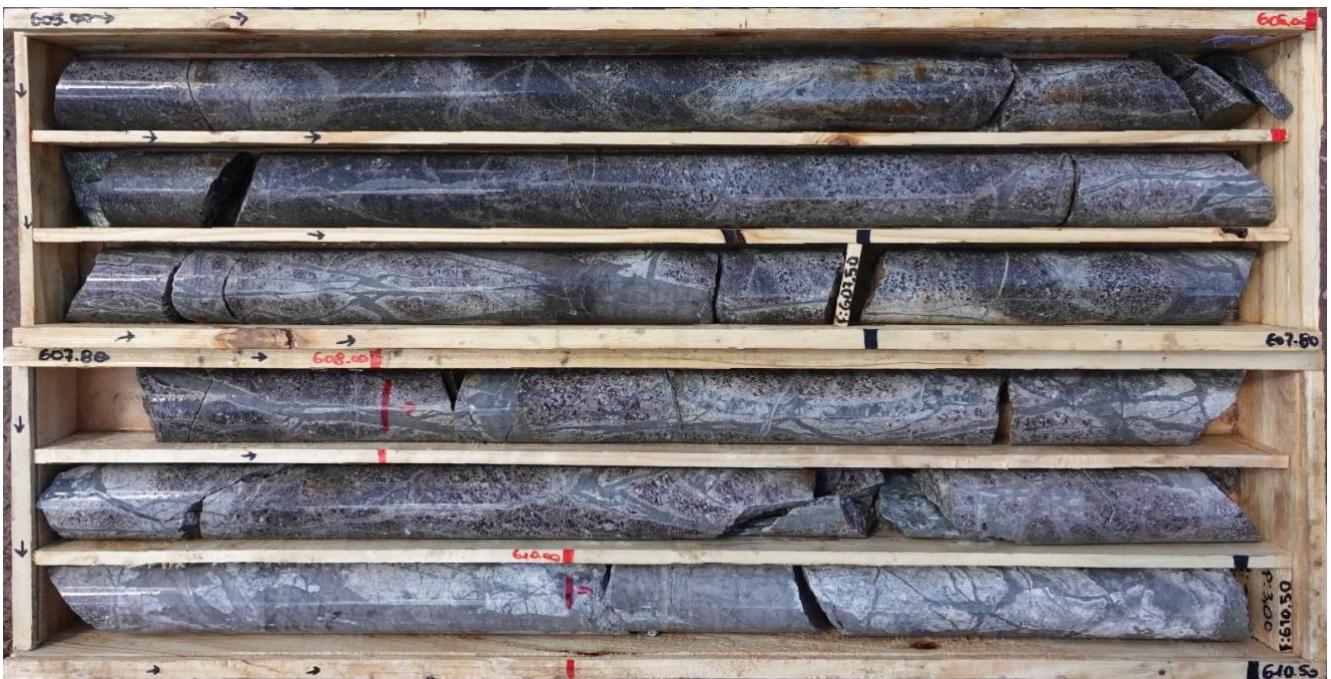
Image 3: PIU-05 605 - 610.5m. Strongly veined and porphyry and diorite host rock, showing multiphase quartz A-veins and associated K-feldspar bearing potassic alteration.
