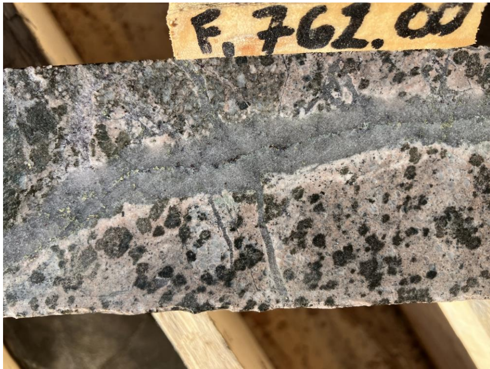
Image 4: A type quartz vein with coarse dissemination of chalcopyrite and bornite associated with intermineral potassic (Kfeldspar-quartz) alteration
