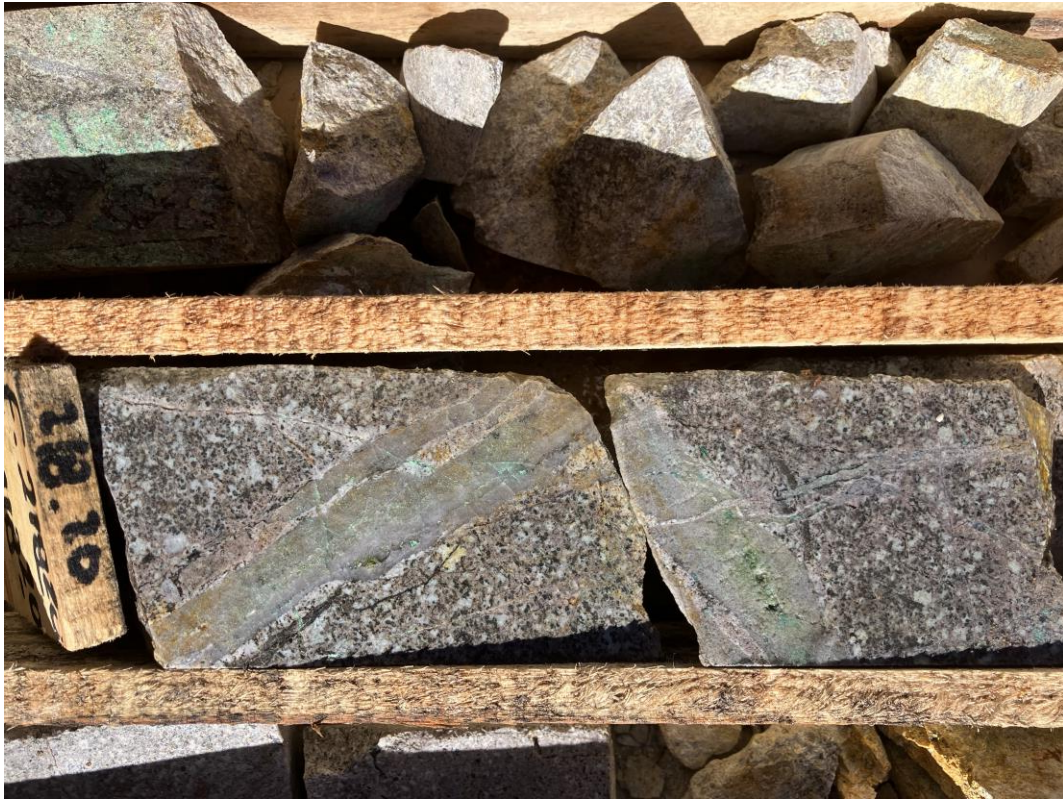
Image 1: Disseminated copper oxides in quartz A-type veinlets overprinting early biotite-magnetite altered quartzdiorite porphyry
