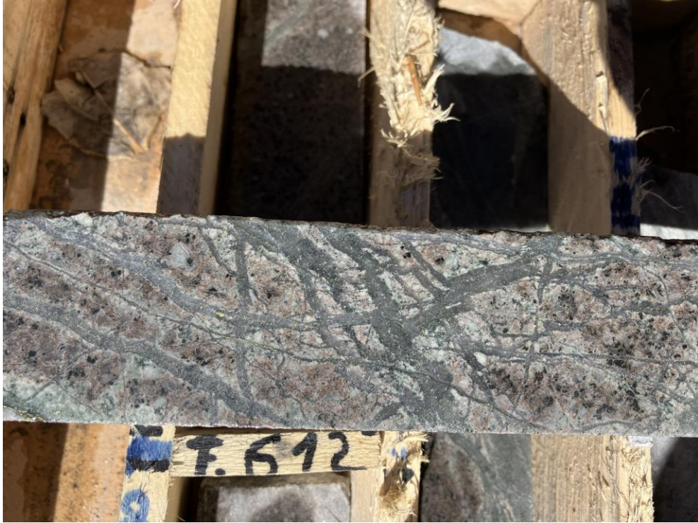
Image 3: Intense porphyry A type quartz vein stockwork with disseminated chalcopyrite and late veins associated with intermineral potassic (Kfeldspar-quartz) alteration
