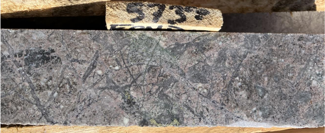
Image 3: Intense porphyry A-type quartz vein stockwork with disseminated chalcopyrite and bornite associated with intermineral potassic (K feldspar-quartz) altered granodiorite porphyry (573m)
