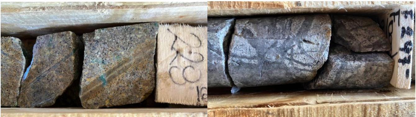
Images 1 & 2: Porphyry qtz stockwork veining with oxide copper mineralization (Left) and supergene enrichment (Right)
