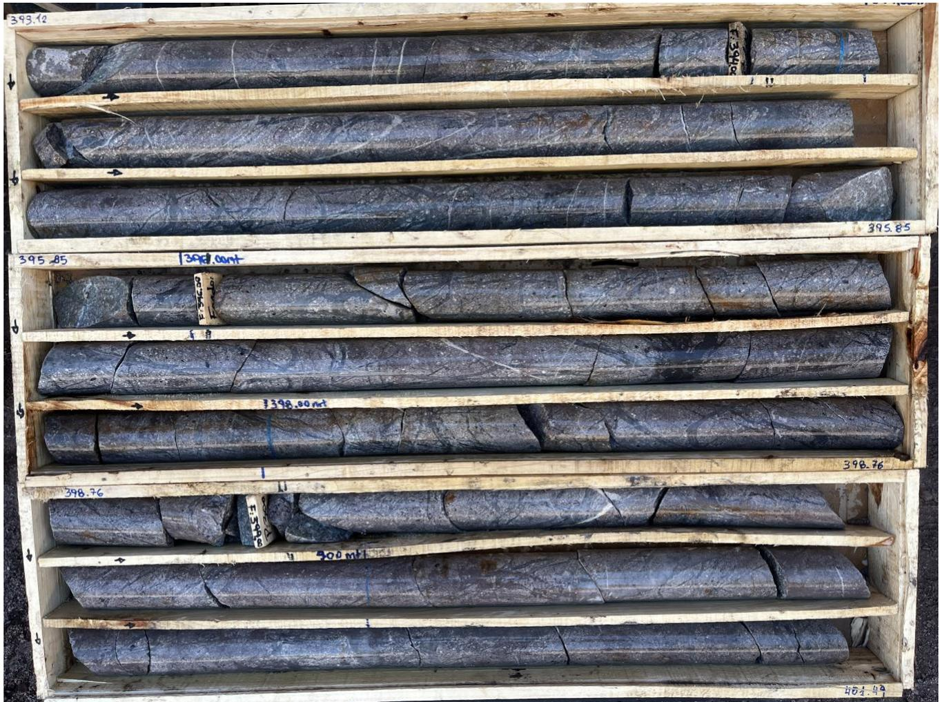
**Image 2: PIU-01 drill core displaying strong Porphyry qtz vein stockworks overprinting potassic altered diorite porphyry intrusion.**
