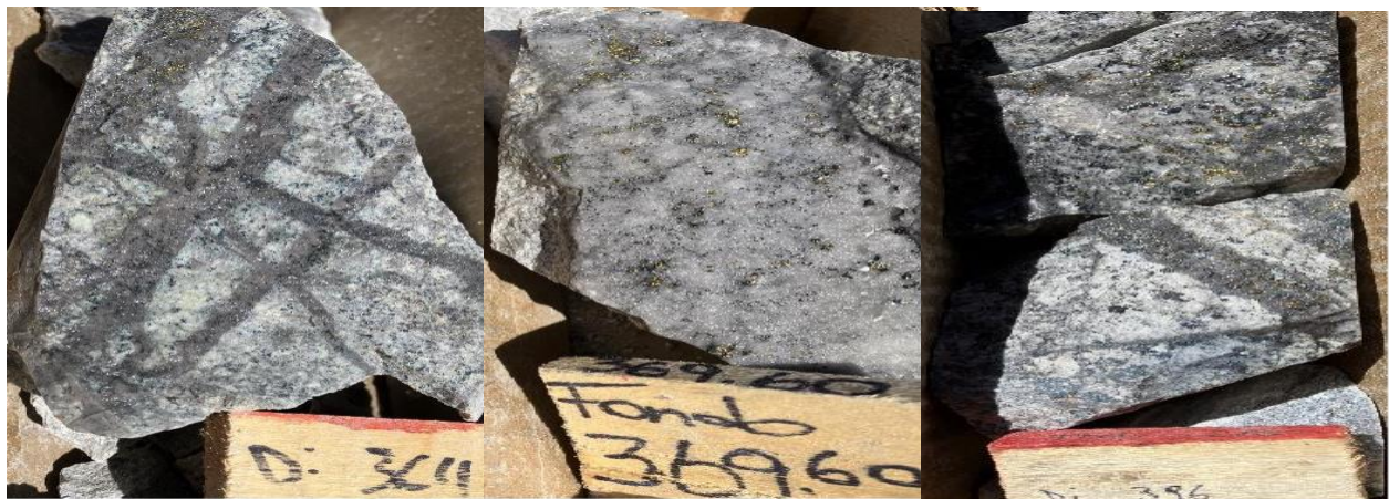
Image 2: A-type quartz veinlet with chalcopryite and some grade of secondary enrichment at PIU16-DDH01
