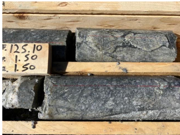
Hydrothermal Breccia with Sulphides and Sericite
