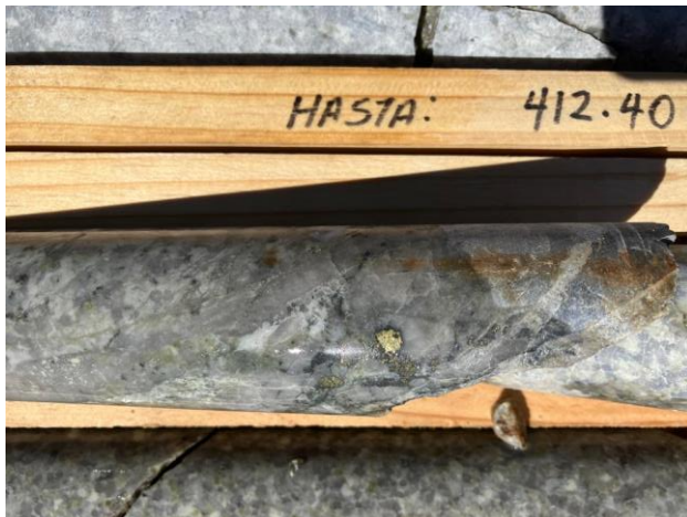
Quartz Vein with Coarse Disseminations of Pyrite-Chalcopyrite
