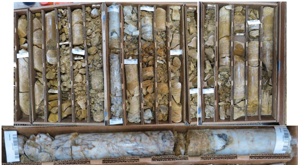
Figure 22. White quartz vein and vein breccia in drill hole 2019-SL-1C (top) and closeup of quartz vein. (Source: CGI)
