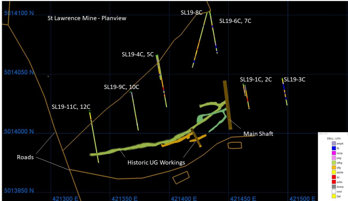
Figure 24. Map of the underground workings and traces of 12 core holes drilled in 2019. (Source: CGI)
