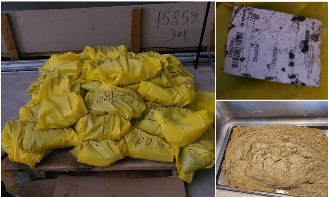
Figure 12.2: Photo of the retained half-samples from the 2022 drilling program at the sample-storage facility during the site visit.
