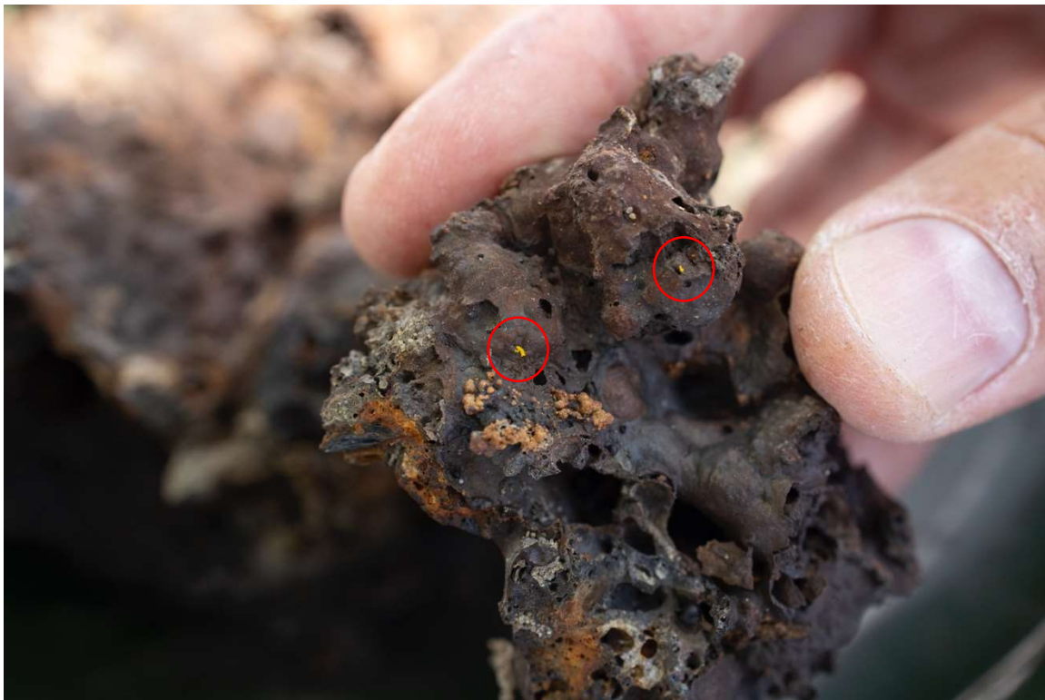
Photo showing visible gold in piece of slag from the riverbed (sample sent to laboratory for assaying)
