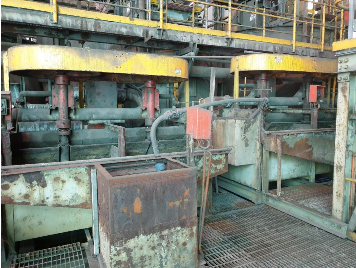
Figure 6-1. Flotation cells at the plant at the Hellyer Gold Mine
