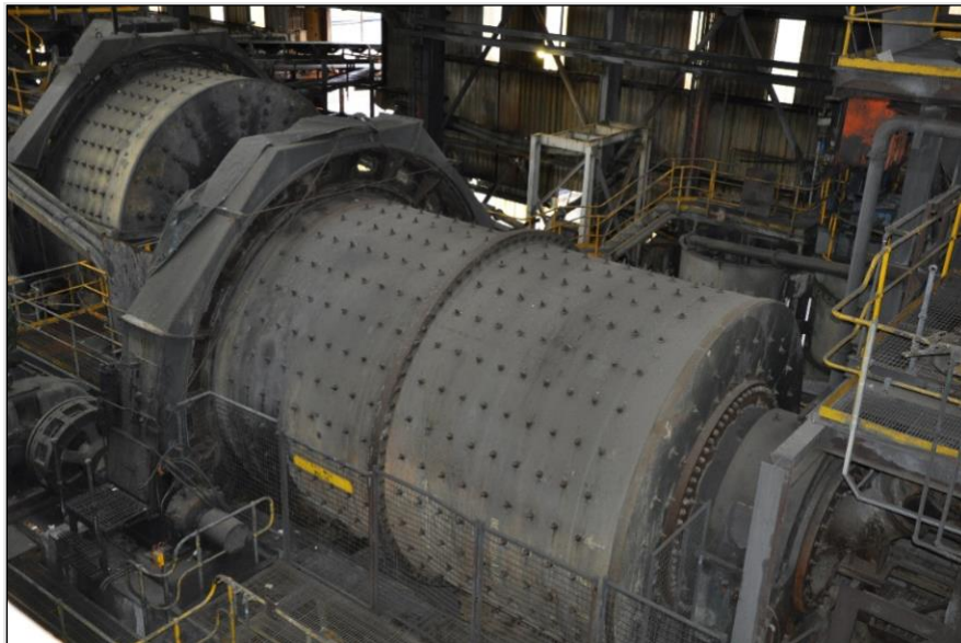
Figure 18-6. View of Hellyer Ball Mill and SAG Mill
