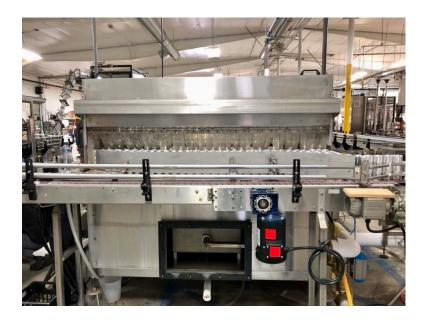
(Caption) The newly validated Tunnel Pasteurizer at Tinley's Long Beach Facility, shown during an aluminum can test, now provides Lakewood co-pack clients with a preservative-free manufacturing option for a variety of still and carbonated product types in both cans and bottles. The Company believes this capability is unique for a licensed cannabis-infused beverage manufacturer in California.
