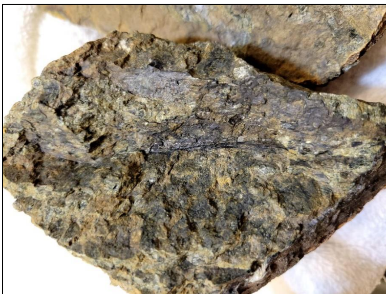
Plate 4 – Sample 534794 – Strongly magnetic, serpentinized Peridotite with mm size magnetite veins (2,106 ppm Ni)
