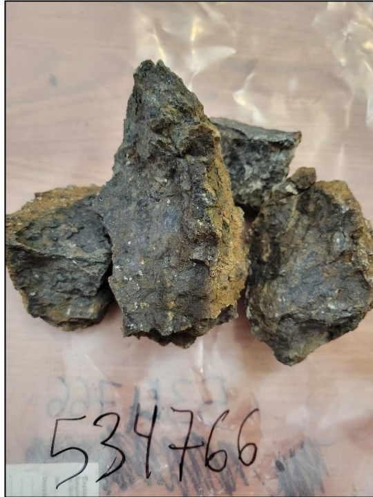
Plate 5 – Sample 534766 – Strongly magnetic, serpentinized, peridotite with mm magnetite veins and potential sulphides
