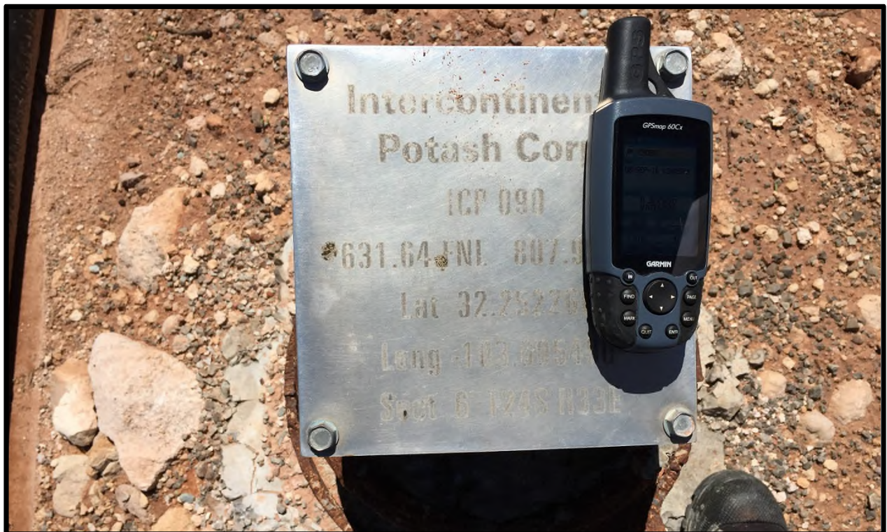
Figure 12.3: ICP-090 Drillhole Collar Monument Visited During QP Site Visit
