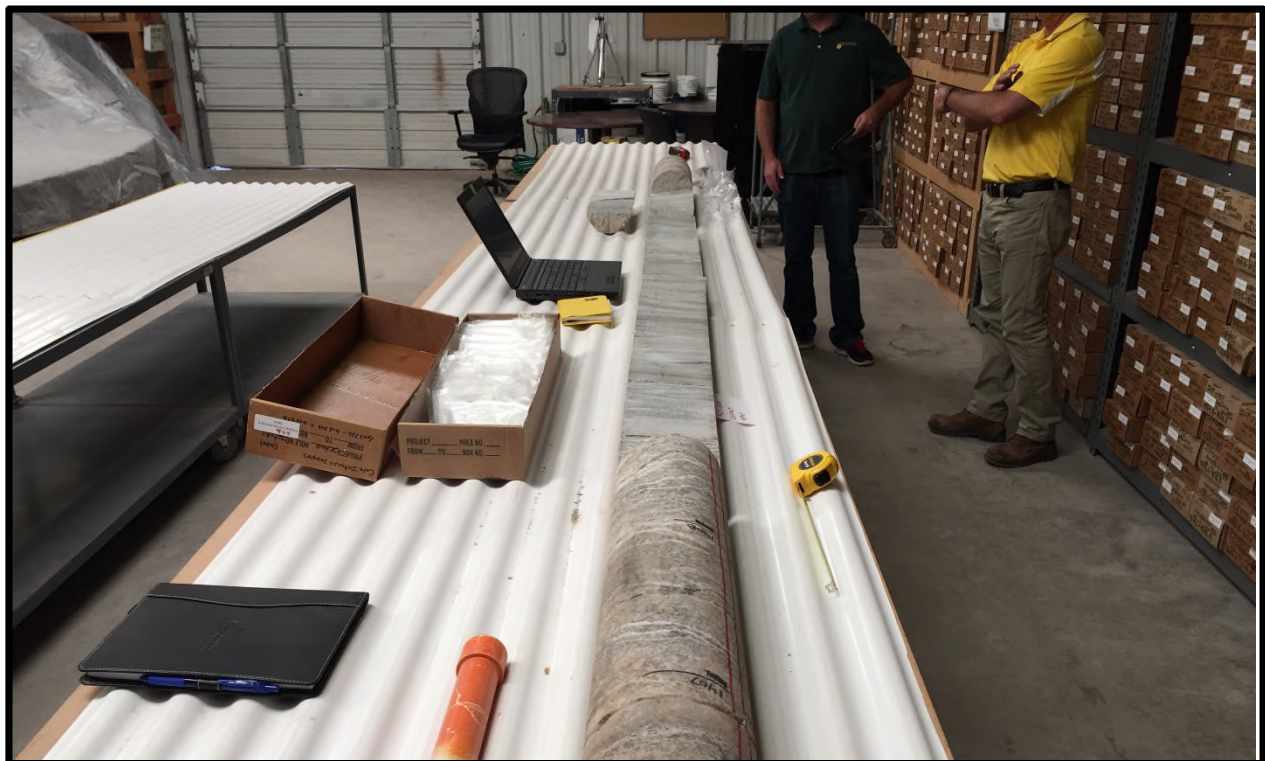
Figure 12.4: Drillhole ICP-085 Laid Out on Core Logging Bench at the ICP Core Facility
