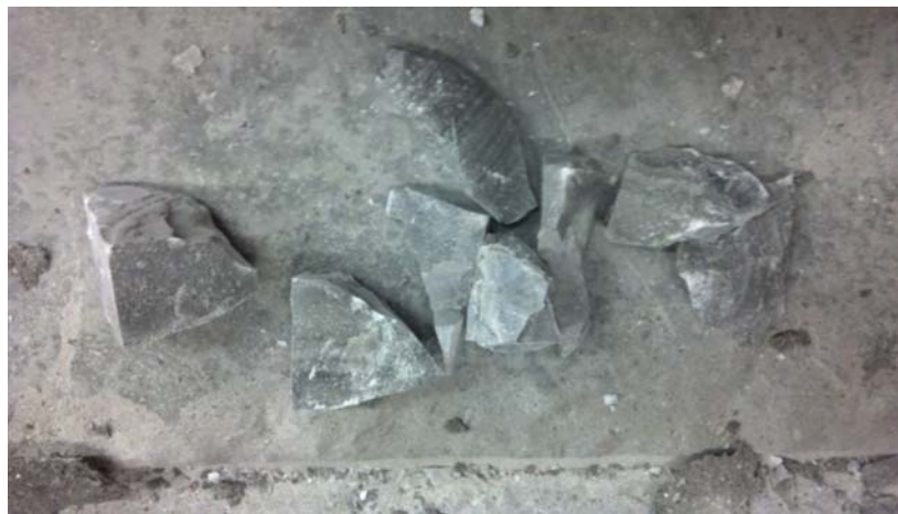
Figure 16-21. Example of Conchoidal Fragments from Cutting Test Run
