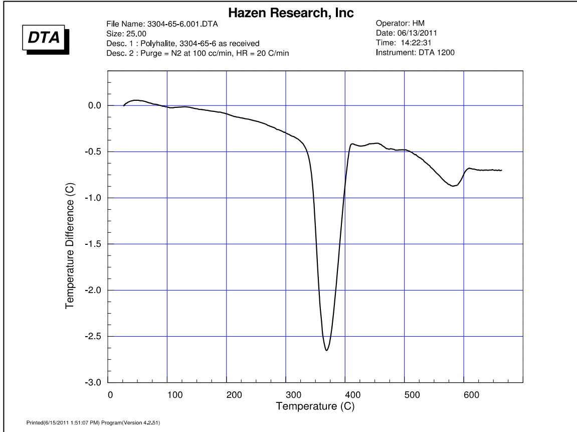
Figure 13-2 Differential Thermal Analysis Scan of Polyhalite
