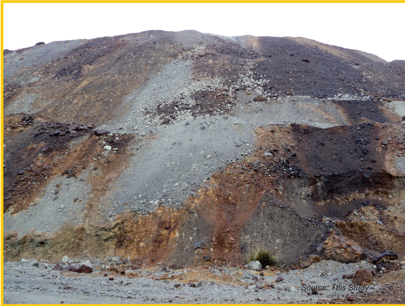
Figure 24. Detailed view of the EMP which consists of various material including altered volcanic rocks, limestones, Pb-Zn mineralized rocks, pyrite-rich rocks, and strongly oxidized rocks.
