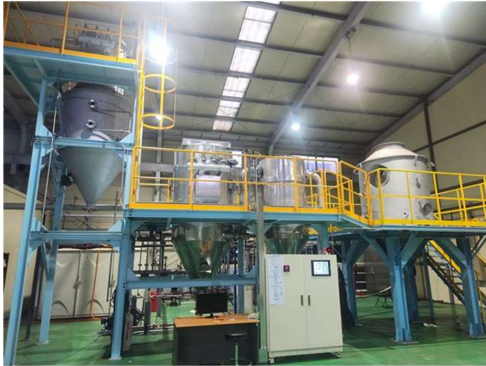
In this picture: Partial view of some of the cyclones and reactor of the 75kW Hydrogen production showcase plant.
