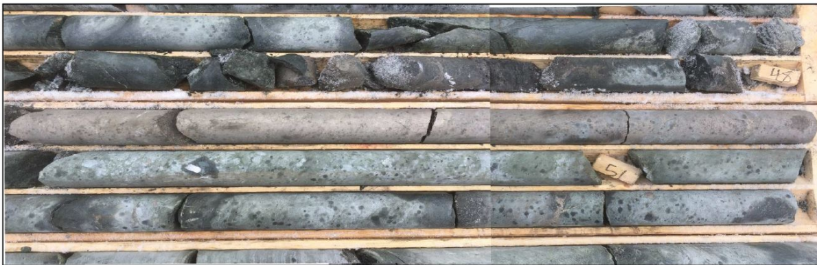
Picture 2. Field Picture of Hole SX-MN21-018 with sections of massive to semi-massive sulphides from 47.5m to 52m.
