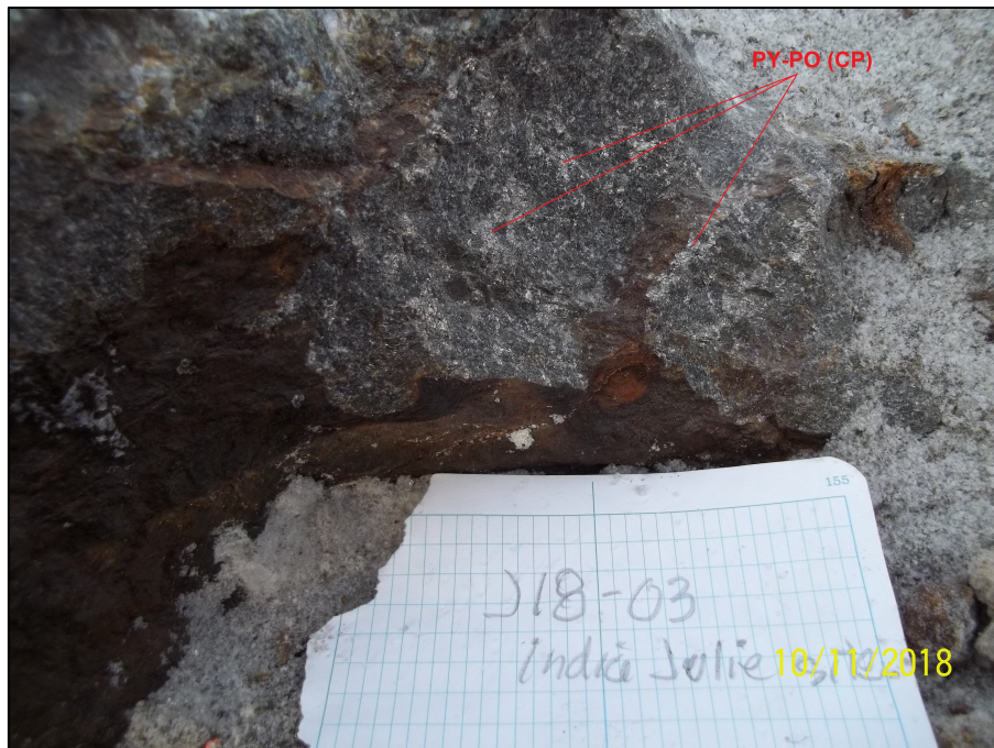
Photo 2: Fresh cut on margin of the drill hole JU-18-03 show fresh pyrite (PY), pyrrhotite (PO), chalcopyrite (CP), and pentlandite (nickel sulfide included in pyrrhotite) stringers and clusters hosted in foliated gabbro-norite.
