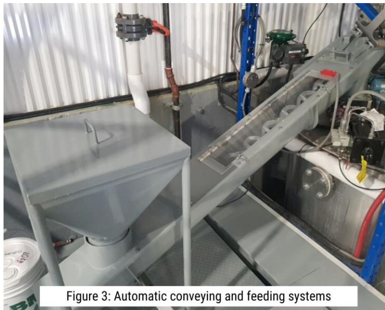
Figure 2: Automatic raw material feeding systems and process control
