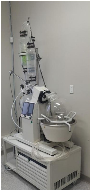
Figure 12: Evaporation equipment for fertilizer by-product trials
