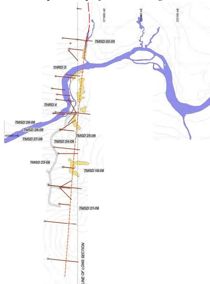
Figure 2: Plan map of Thor project with drilling and vein intercepts.
