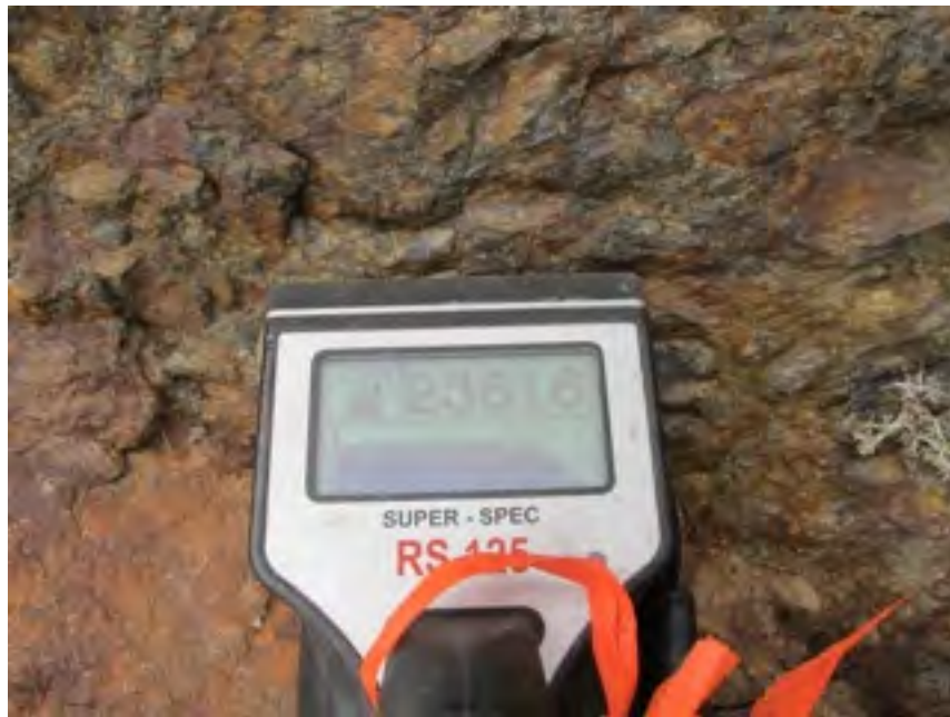
Figure 21: Richore Conglomerate. Anomalous radioactivity (23,616 cpm) from rusty pyritiferous quartz pebble oligiomictic conglomerate, Richore Occurrence, south pit.
