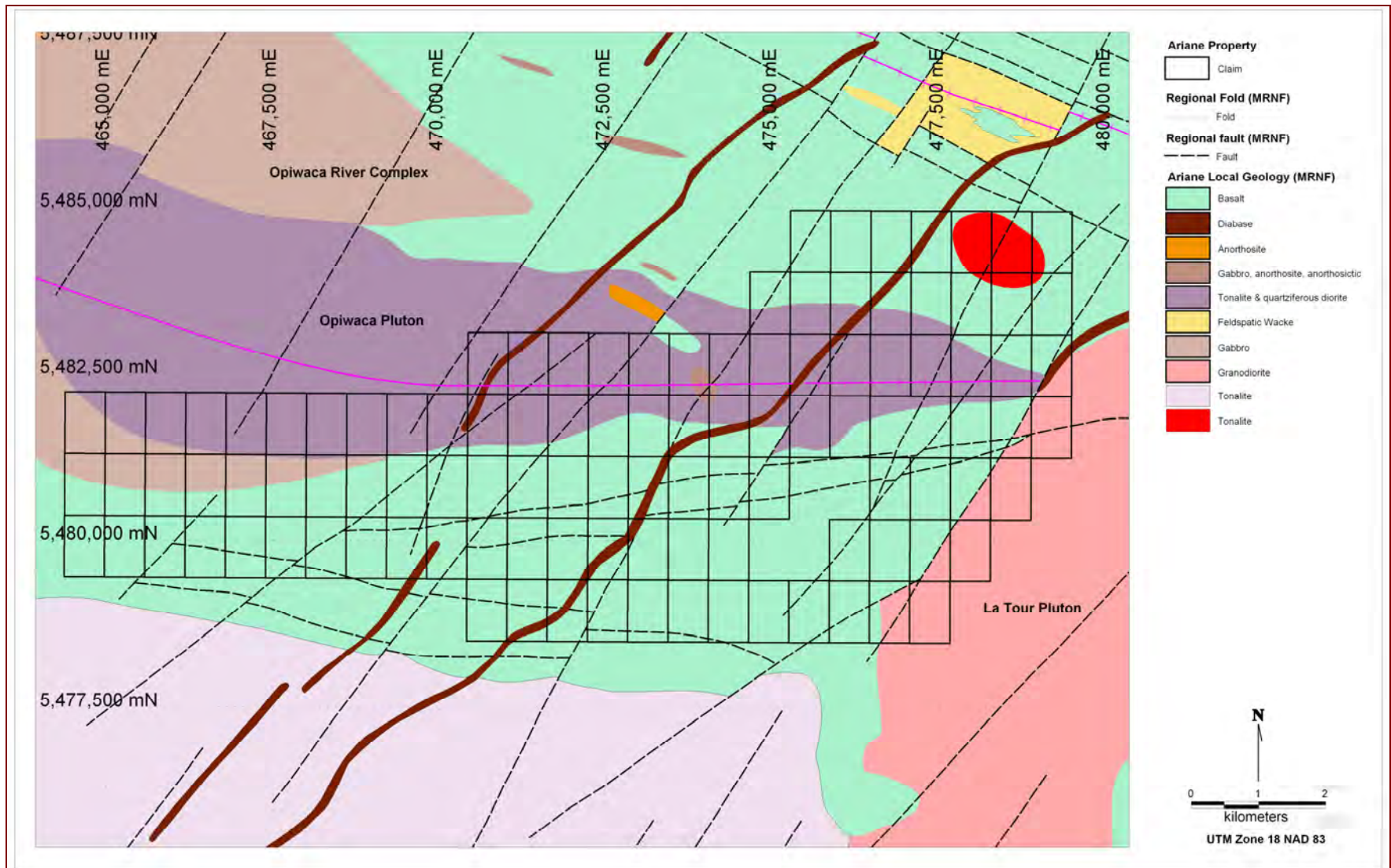
Figure 9: Geological map of the Ariane property showing Archean Obatogamau basalts interstratified with metasediments, in contact with syn-tectonic tonalite and gabbro and crosscut by late Kenoran granodiorite.
