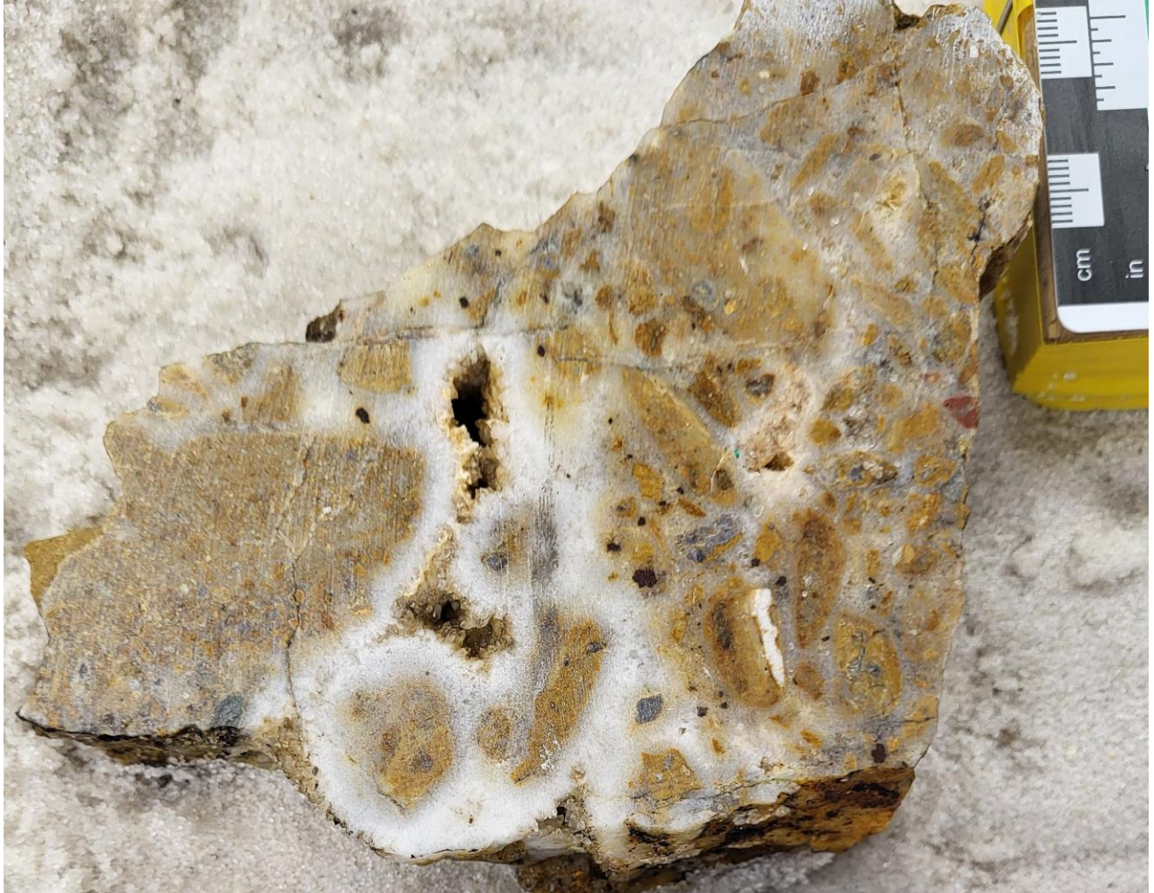
Image 2. Slabbed grab sample from locality shown in Image 1, of quartz vein breccia cementing altered volcanic rocks from the western part of the B&C Springs property.
