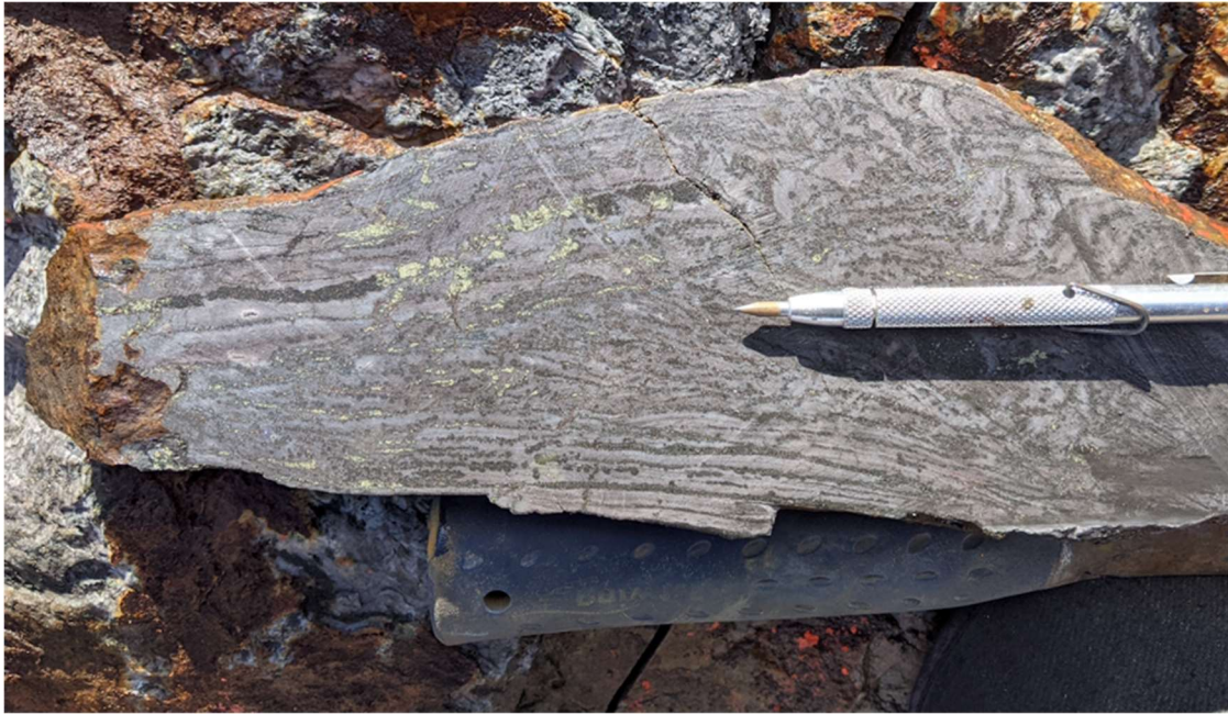
Visible Copper in Cut Channel Sample
