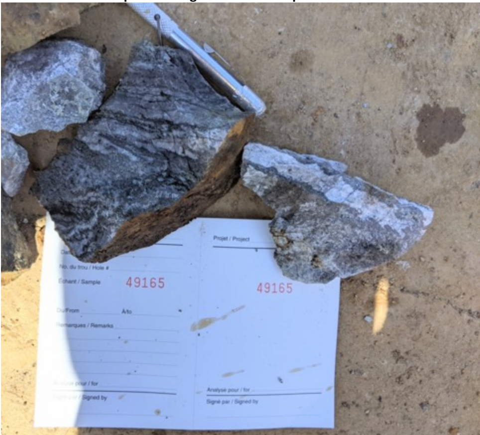
Mineralized Fine Sulphide Stringers in Grab Sample
