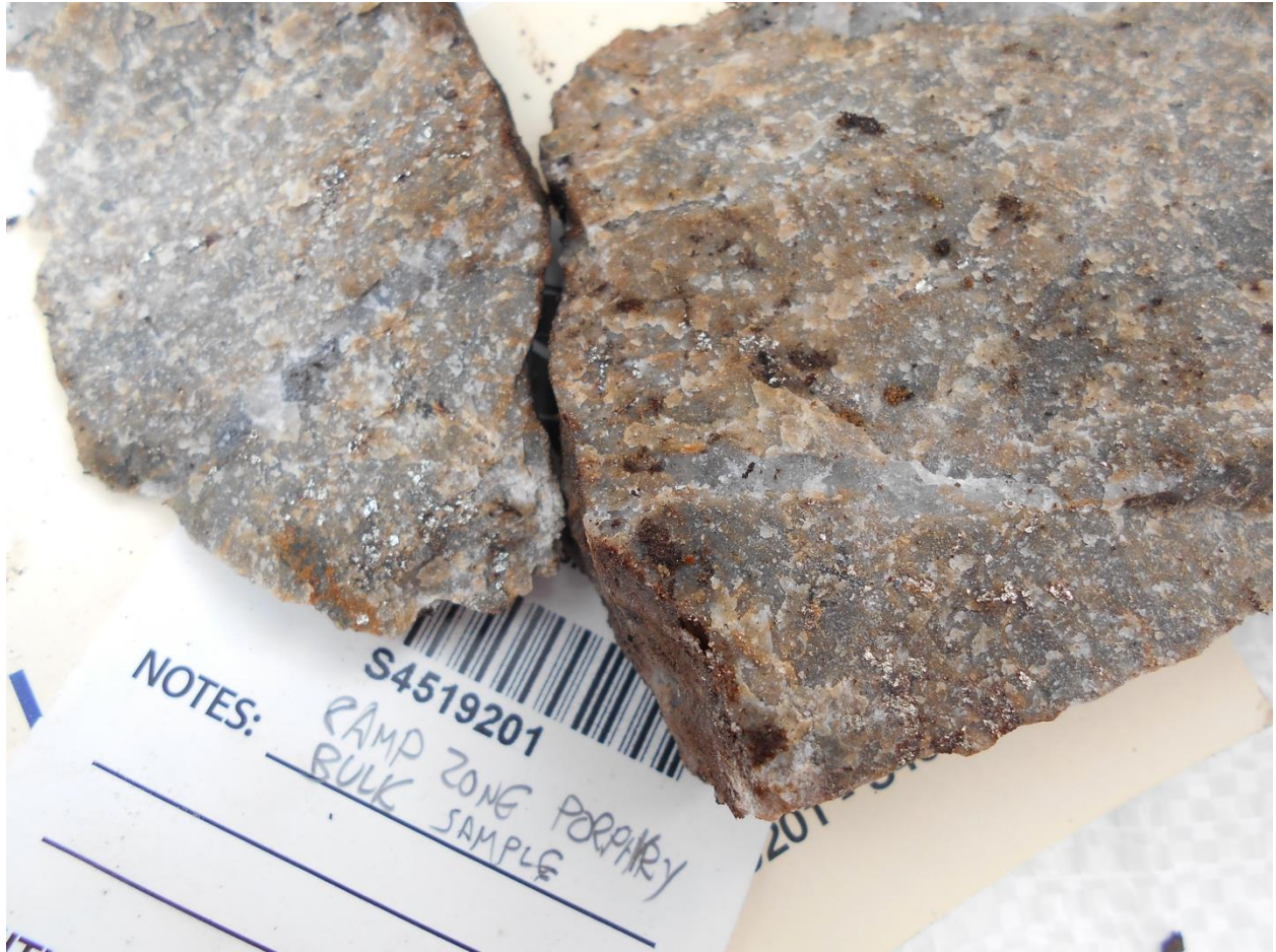
Photo 6: Example of the porphyry zone showing sulphides in halo around quartz veins, from 2015 surface work
