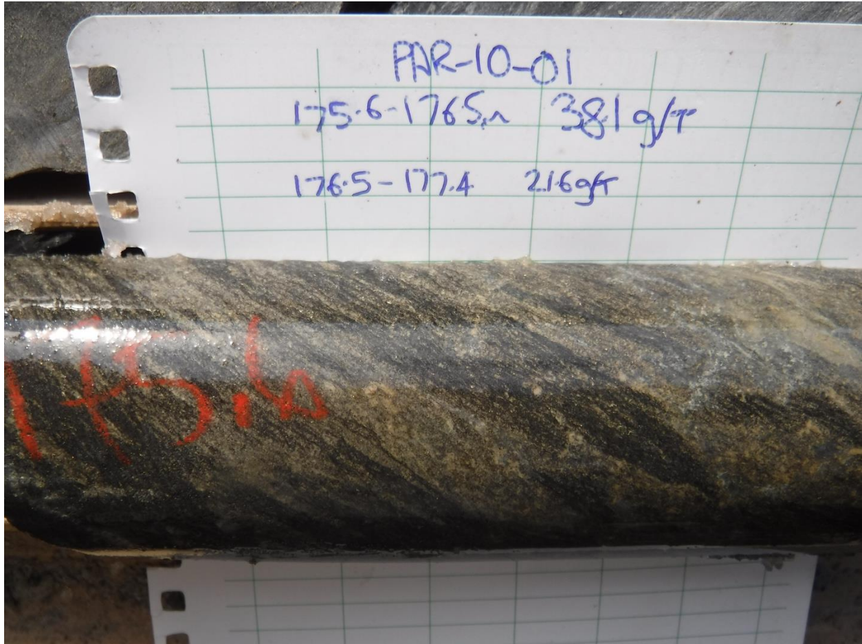
Photo 5: Example of Tuff Zone, showing biotite and fine sulphide mineralization, from 2010 Savant drill core
